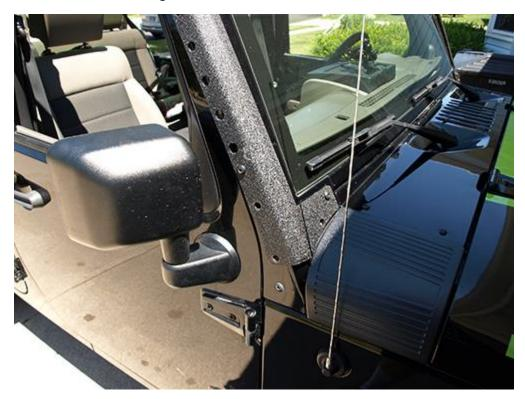
**Note:** If installing the Windshield Double Row Light Bar Mounting Bracket by yourself. Tape a rag around the end of the Light Bar Bracket that will be secured to the Driver Side Bracket. The rag will help prevent damage to windshield.
