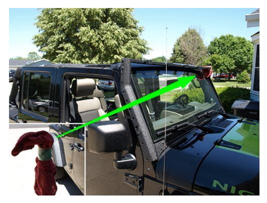
6. Secure the Light Bar Bracket to the Driver Side Bracket using the last two (2) of the supplied M8x20 Hexagon Bolts. Do Not tighten all the way.
