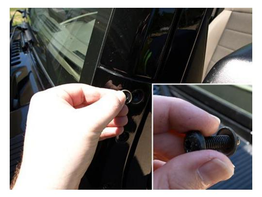
3. Place the Driver Side bracket on the driver side of the Jeep. Secure the bracket using the factory TORX T40 bolts. Do Not tighten all the way.
