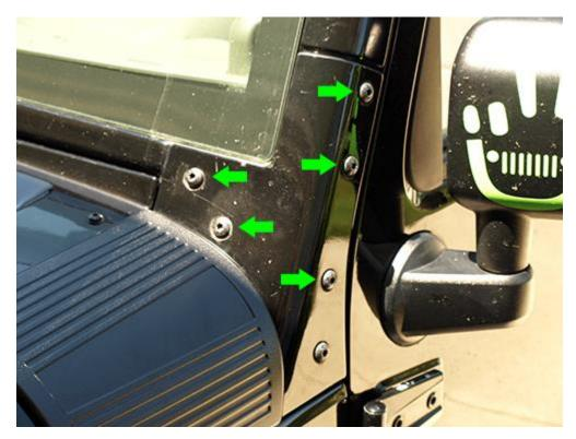
2. Remove the plastic washers if they come off when removing the TORX T40 bolts. Place the plastic washers back in to the windshield bracket holes.
