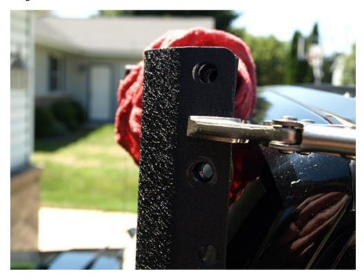
7. Secure the Passenger Side Bracket with the last three (3) factory TORX T40 bolts. Tighten all bolts on passenger side and driver side.
