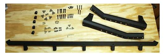
**Note:** This Installation guide is to show you how to install the DV8 Off-Road Windshield Double Row Light Bar Mounting Bracket only. The lights will determine which nuts, bolts and washers will be used to secure them to the light bar mounting bracket.
