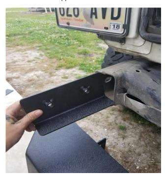
5. (An extra pair of hands here will help) Lift bumper into place and using the supplied bolts and washers from DV8 begin all 4 bolts to hold the bumper in place using the 16mm socket and ratchet.
