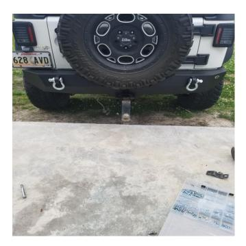
7. The kit comes with a spacer that may or may not be needed, here is an example of where it would go in between the bumper and frame where a OEM tow hitch would go. Some need it, others do not. The supplied hardware comes with the bumper.
