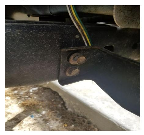
2. Using the 19mm socket and ratchet, remove the 2 bolts (1 on each side) holding the top of your bumper on.
