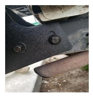
6. Using the second pair of hands or your body weight make sure the bumper is pushed all the way up and into place then start tightening all 4 supplied bolts using the 16mm socket and ratchet.
