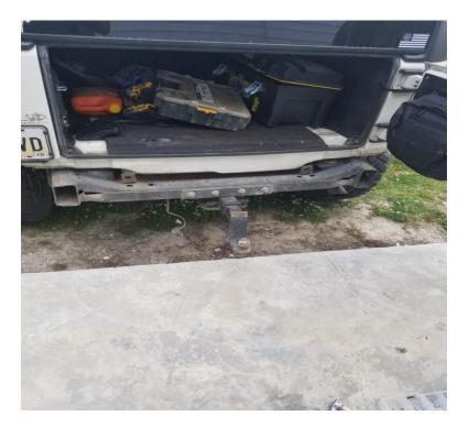
4. Place the supplied brackets into the rear frame openings as a mounting point for the new bumper.
