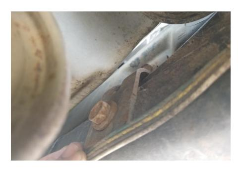
3. Pull off your rear bumper from the frame. At this point, if you have a tow hitch, remove it using the same 19mm socket and ratchet.
