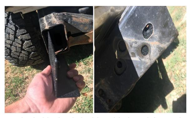
• Place 4 long bolts with a washer through the same holes where your hitch was secured.
