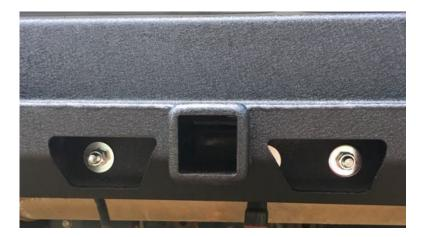
Once secured, go to the sides and fasten the bolts to the frame rail with a washer against
