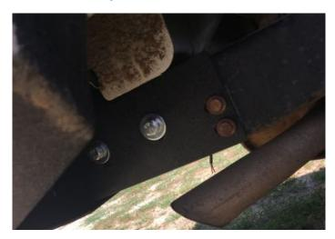
• Once the bumper is fully secured, trim length as needed from spliced wires and connect to the red and black wire on the light pods – red to red and black to black. Use zip ties to secure wires.
