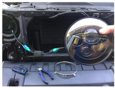
4. Place the original bezel over your new headlight and position the headlight back in the housing. For proper placement, ensure that the smaller LED is on top and the larger LED is on bottom. Reinstall the bezel screws, and grille.
