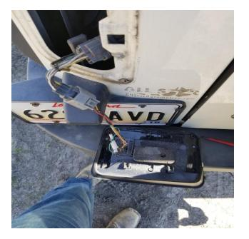
4. Place new DV8 Off-road Taillights appropriately and screw back in using stock Phillips head screws.
