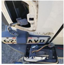
3. Plug in the connector to the new DV8 Off-road Taillights.
