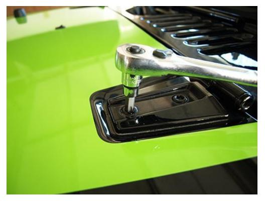
2. Place the Hood Light Bar Mounting Bracket on the hood brackets. Place two (2) TORX T50 bolts on one side and then two (2) on the opposite side.
