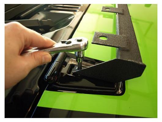
Note: Depending on your TORX T50 socket you may need to use an extension to secure the bolt that is closest to the metal bar of the bracket as shown below.
