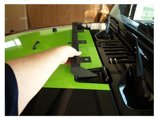
3. Tighten all four (4) TORX T50 bolts securing the Hood Light Bar Mounting Bracket to the hood.
