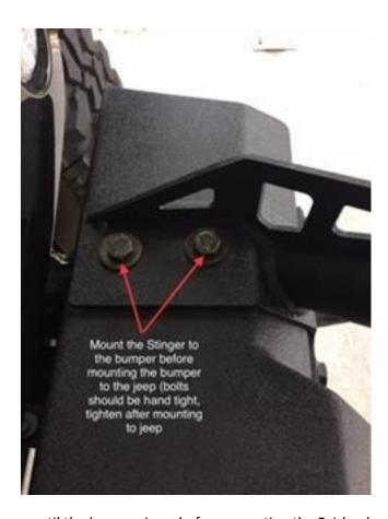
until the bumper is on before mounting the Fairlead mounting plate.
