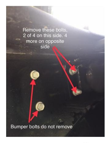
outer nuts, there are two more on inside of frame; repeat on both sides.
