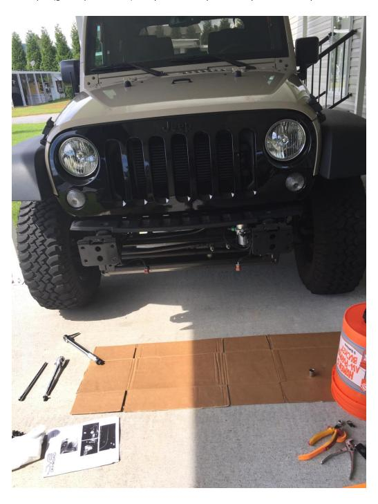
7. Since your new bumper came in 3 pieces, there is some simple assembly required before mounting the bumper to the jeep. The Stinger must be mounted to the top of the bumper before putting the bumper/Stinger on the jeep. Hand tighten these 4 bolts (2 on each side) and finish tightening after bumper is mounted. You can wait
