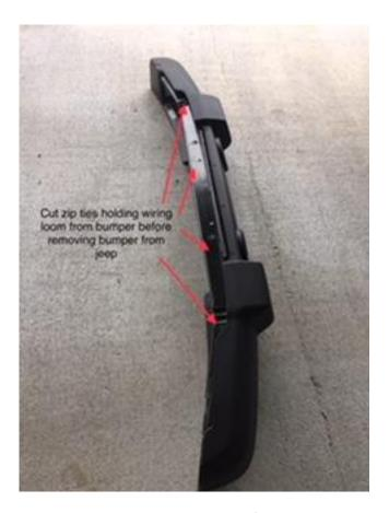
4. Cut the zip ties that are holding the fog light wiring loom to the stock bumper.
