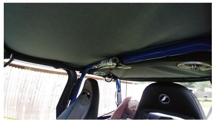
6. After snugging the first clamp with the correct orientation, install the 2<sup>nd</sup> clamp
