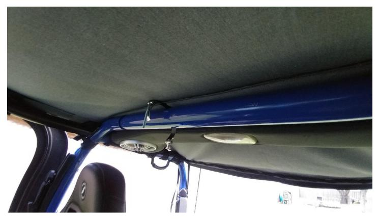
5. Use a 11 mm socket to snug up the clamp to hold the mount in place
