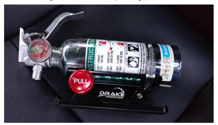
4. Using the 2 ¾" hose clamp tighten down the fire extinguisher
