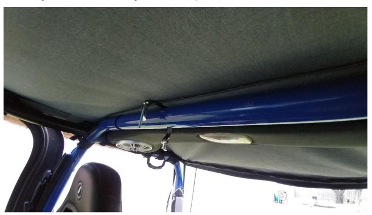
8. Use a 11 mm socket to snug up the clamp to hold the mount in place
