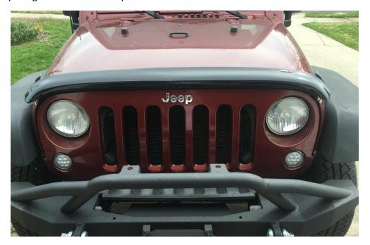
2. Begin to unscrew the six screws that hold the grille onto the Jeep.
