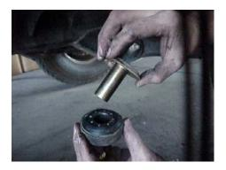
7. Insert stock steel inserts inside top portion of body lift spacer (Note: It fits tight, you may have to use a vise.)
