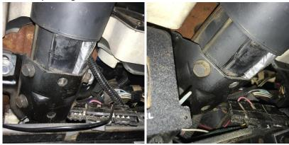
20. Reattach the three screws that hold the turn signal switch in place. I had to rotate the switch to access one of the screws.
