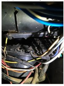
17. Attach a guide strap to the wires. Remove the turn signal switch and gently pull the wires and guide strap up through the steering column. (The guide strap is a recommendation based on my mistake and then spending three hours trying to fish the new harness down the column.)
