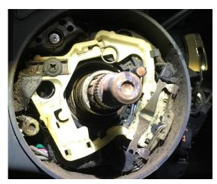
14. Remove the turn signal switch retaining screw. This will release a linkage between the turn switch module and the turn signal arm.
