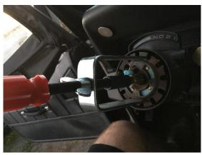
11. Use a pick or couple of small screwdrivers to move the retaining clip up on the center bolt. Remove the compressor and then the retaining clip.
