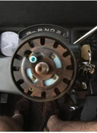
10. Attach a compression tool on the center bolt and tighten to compress the locking plate away from the retaining clip. The official service manual strongly advises to not try and remove the retention clip without using a compression tool.
