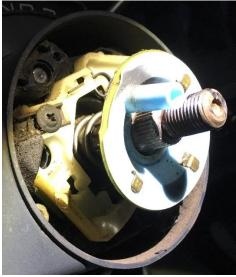
13. Remove the three Philips head screws that hold the turn switch module in place. You will need to move the turn signal to access one of the screws.
