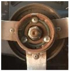
4. Remove Bushing and Receiver. These are held in place three Phillips head screws.
