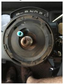
9. Use flat head screw driver to pop lock plate cover off. Gentle outward pressure at each of the slits will move the cover off.
