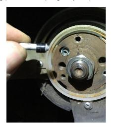
7. Remove steering wheel retaining nut with 5/8 socket. Mark center bolt and steering wheel with a mark for alignment during reassembly.
