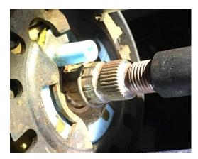
12. Remove the lock plate, cancelling cam, preload spring, and thrust washer.
