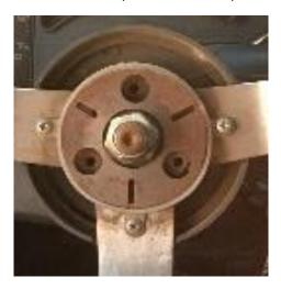
5. Remove flex-plate and insulator. The insulator is held to the steering wheel with three Phillips head screws.
