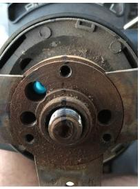
8. Bolt a steering wheel puller to the steering wheel. Many chain auto parts stores have pullers as part of their tool loan program. Tighten the center bolt on the puller and the steering wheel will come loose.
