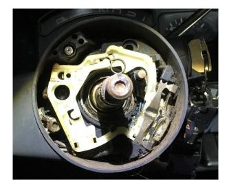
15. Remove the hazard-warning switch. It is held in place with one Phillips head screw.
