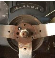
6. Remove the horn contact and spring (note order: spring deepest, pen, retaining ring holds pen in place).
