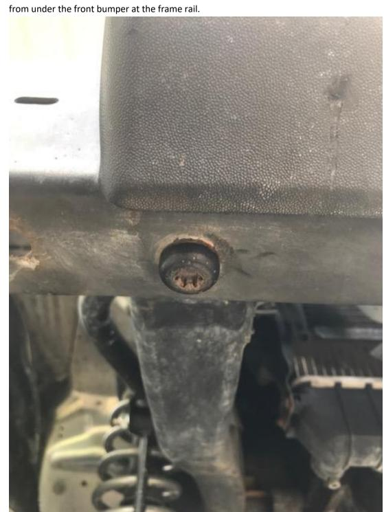
1. Remove the OEM front bumper by removing two T55 Torx socket head bolts (1/2" X 1 3/8") from under the front bumper at the frame rail.
