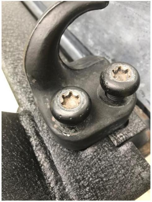
9. Torque all four top T55 bolts and two bottom T55 bolts to OE specifications.
