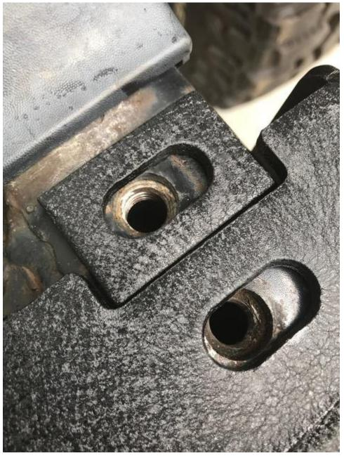
8. Install the tow hooks and four T55 Torx socket head bolts (1/2" X 2 3/8") into the top of the front bumper.
