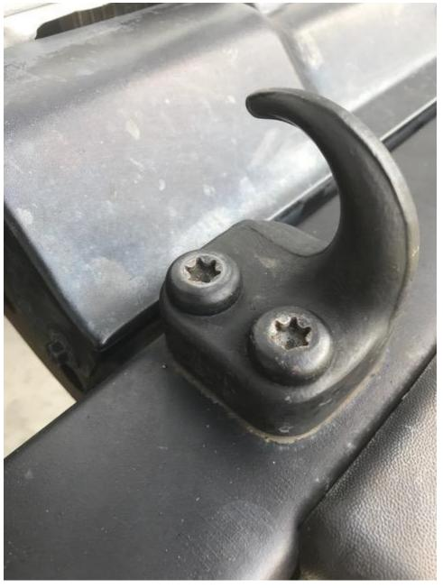
3. Retain OEM bolts and tow hooks for reuse.
