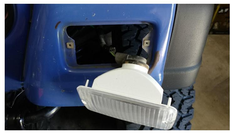
9. Use the pins to line up the light housing with the fender and install the 2 - T15 star bit screws
