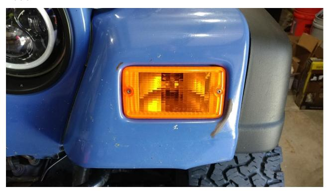
2. Remove the 2 - T15 star bit screws
