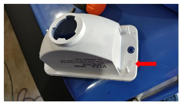
8. Insert the bulb socket turning it counter clockwise
