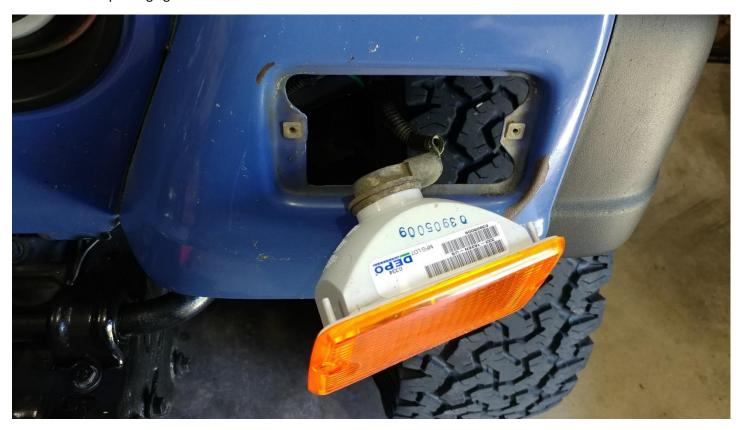
4. Twist the light socket clockwise and pull out
