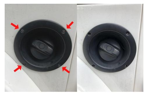
3. Place Locking Fuel door over factory gas housing and line up the screw holes.
