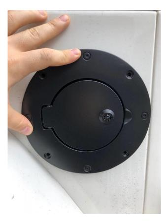
4. Use the Torx key to install the torx screws in the corresponding screw holes.
