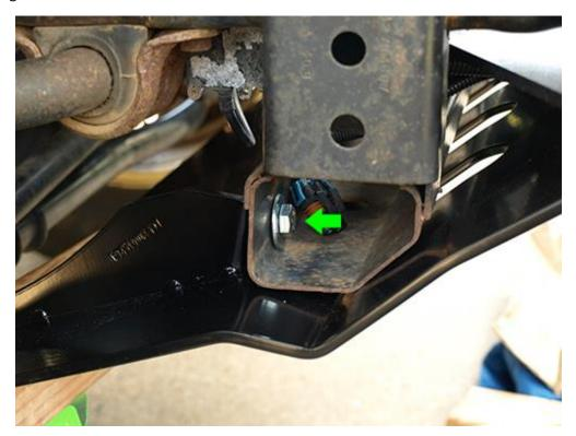
7. Drill a hole up to 9/16 in size on the bottom frame brace of the passenger side. Mark the location with a Center Punch. **NOTE:** Recommended to us a small drill bit to make a pilot hole and work your way up to the 9/16 drill bit size. You may need to remove the front skid plate when drilling the hole.
