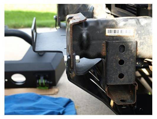
5. Lift the front skid plate, using a floor jack or other device, until the bolt holes of the welded bracket are aligned to the bottom frame brace.
