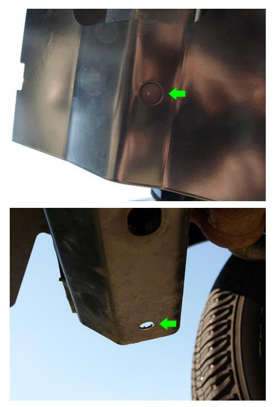
8. Place a larger washer (provided) onto an 18mm bolt. Slide the bolt through the hole that was just drilled into the frame brace. Place an additional washer on the other end of the bolt and a 19mm nut. Tighten the bolt.
