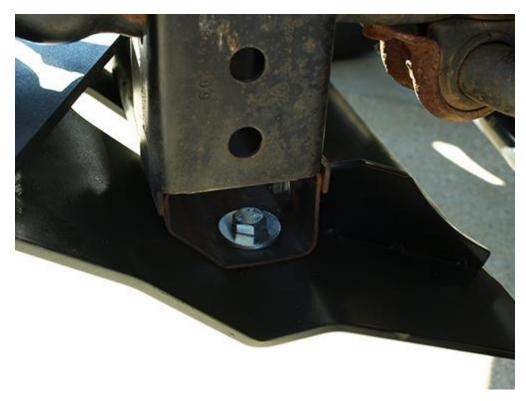
10. Reattach your front bumper, tighten all bumper bolts and reconnect the fog light wires. **Important Note:** *Depending on the bumper style you may need to remove the top front bolts that are holding the front skid plate to the frame that were installed in step 4.*
