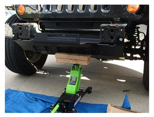
Slide a small washer (provided) onto a 16mm. Slide the bolt through the bottom frame brace on the passenger side and through the front skid plate. Secure it in place with a 17mm nut. Repeat this step on the driver side. Loosely tighten the bolts.
