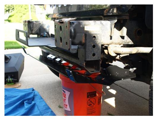
4. Slide an 18mm bolt through the front hole of the skid plate on the driver and passenger sides, attaching it to the frame of the Jeep<sup>®</sup>. Place a 19mm nut onto each bolt. Loosely tighten the bolts.
