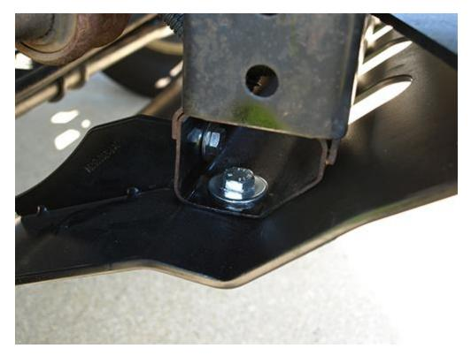
9. Repeat step 8 on the driver side and then tighten all bolts that are holding the front skid plate to the frame brace.
