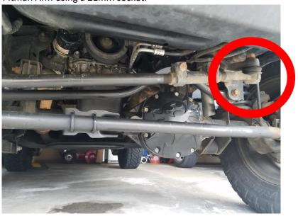
2. Hand screw the nut back on a few turns, so that when it drops (step 6) it will not fall on you or the ground.
