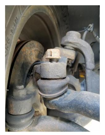
4. On the knuckle, use a hammer to strike the metal.
