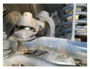
6. The pitman arm connects to your steering box, so you want to be careful. Put a hammer on the backside of the metal and strike it with the other hammer. You will know that you are doing it correctly if you strike with one hammer and the one on the backside comes off (you'll feel it). This will help transfer the energy of the strike and protect the steering box.
