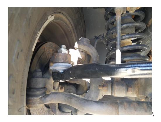
12. Make sure your steering wheel is centered. Adjust the sleeve as necessary and then tighten the 2 adjusting sleeve bolts with the threads facing backwards using a 15mm socket to 26 ft-lbs
