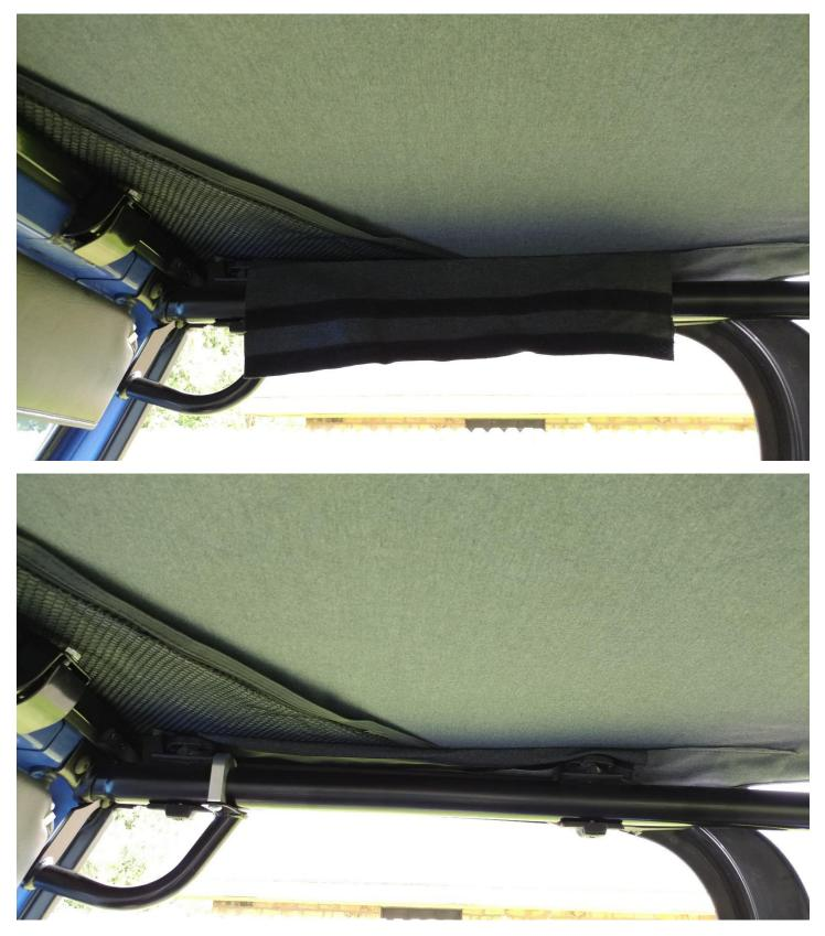
9. Secure the two straps around the center roll bar
