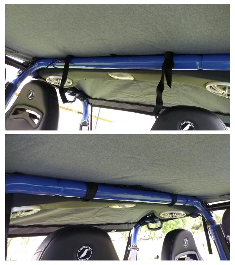
10. Secure the outer straps around the center roll bar
