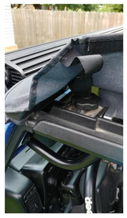
7. When using the door surrounds clip the plastic portion into the channel just like the factory soft top.
