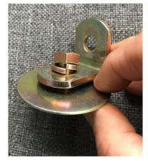
7. Attach the seat belt buckle to the L bracket with a spacer and lock washer on the bolt side. I did not have enough clearance on either side to use a socket driver and thus had to use two 11/16 wrenches. Align the buckle to fit your desired location with respect to the seat and then tighten the bolt and washer.
