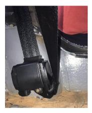
5. Remove the original seat belt buckel from the jeep tub using the T45 socket. A plastic cap covers the bolt.
