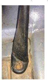
6. Bolt the "L" bracket to the tub of the jeep in place of the old bracket. I used the large washer below the bracket and a shorter bolt provided in the kit along with a lock washer. One end of the "L" is slightly longer than the other. I used the shorter side on the tub and longer side on the seat belt clip. (The L may be reversed in this picture.) I found this configuration gave the best clearance for the seat belt buckle to pivot. Tighten bolt to tub with 11/16 socket.
