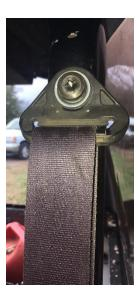
2. Remove the lower seat belt assembly (retractor end) by removing the T45 bolt from below the assembly. I found a socket extension was very helpful.
