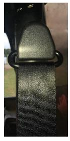
4. Attach the lower seat belt assembly and the end of the belt to the jeep tub where you removed the old assembly. I reattached mine with the original T45 bolt, but a new bolt is provided in the kit. If you use the bolt in the kit, it is the longer of the two bolts. Unlike the original retractor, this belt does not need to be vertical to retract, but you should strive to align it as vertically as possible.
