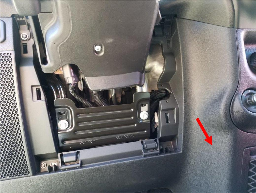
9. Using a phillips screwdriver and the supplied screws, install the microphone hanger. Be careful not to overtighten or you could strip out the plastic. *Note: It is a good idea to replace these screws with nuts and bolts, because the plastic can strip very easy.*
