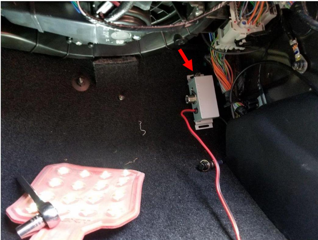
3. Remove the plastic piece inside the passenger door jam. This can be done with your hands, or gently with a flathead screwdriver. Then route the black and red power wires up through this panel.
