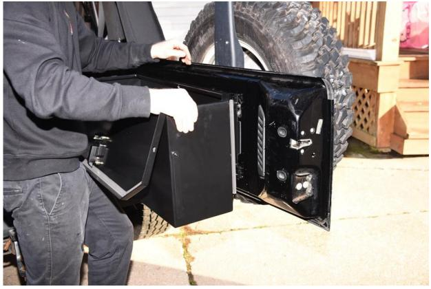
6. Take correct Allen bolt and circler washers, then tighten box to bracket with 5/32 Allen Key. There will be 8 bolts and holes. May help to have extra set of hands to hold box while you tighten.
