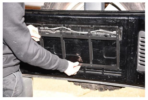
3. Using 5/64 Allen key and correct Allen bolt, tighten locking bracket to top mounting bracket. Repeat for all 4 locking brackets.
