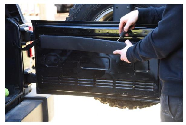
2. Place bottom of mounting bracket into tailgate slot. Should be placed in top bottom slots, with one slot skipped in middle.
