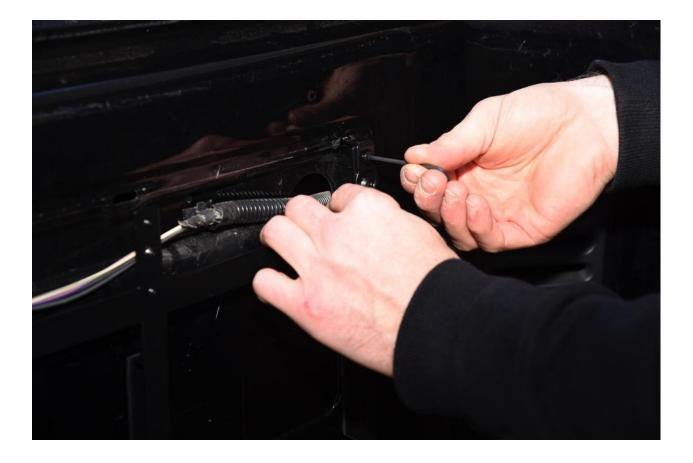
4. There will be rectangular washers and bolts. Tighten rectangular washer to lower mounting bracket with 5/64 Allen key and Allen Bolt.
