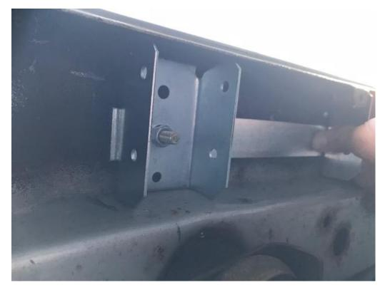
3. Remove brackets and center punch markings on body metal.
