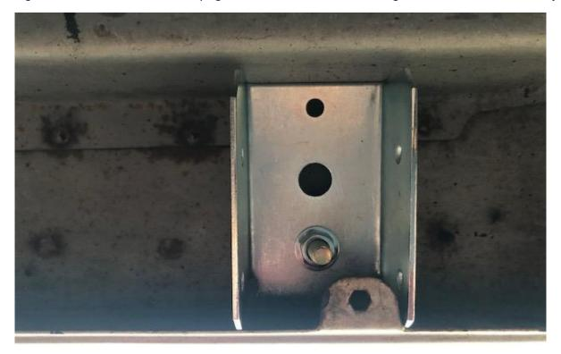
8. Hand tighten bracket bolts and washers to the steps using the image below.
