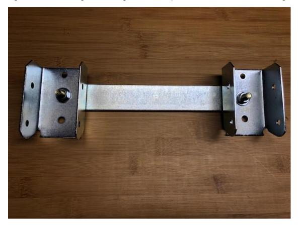
2. Hold brackets flush with the body metal in desired position beneath door entry. Mark the outermost bracket hole with a pencil (Not the center hole).
