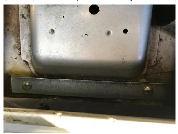
7. Using a 13mm socket wrench securely tighten bolts and washers to carriage bolts from underneath the jeep.
