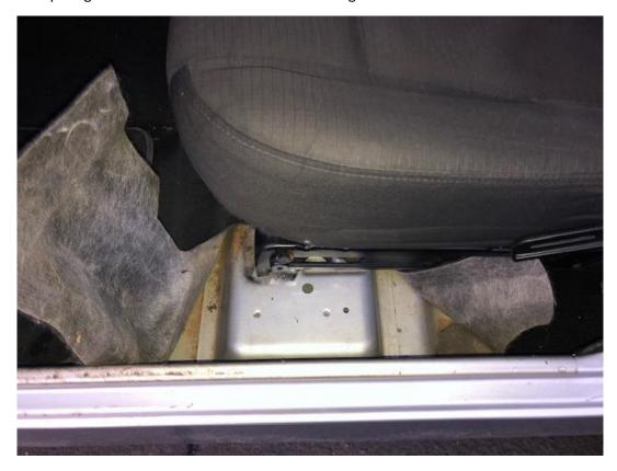
5. Using a 5/16" drill bit, drill through the two center punched holes from the underside of the Jeep.
