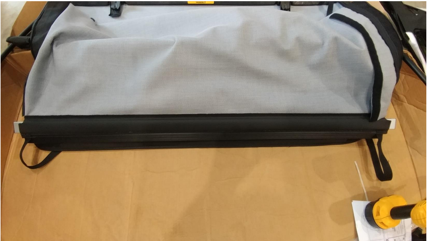
30. Lay the soft top onto the Jeep and secure the sun rider bars. Line them up and pull inward on the cone shape
