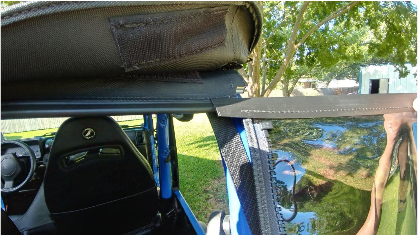
37. Slide the tailgate bar along the bottom side of the rear window
