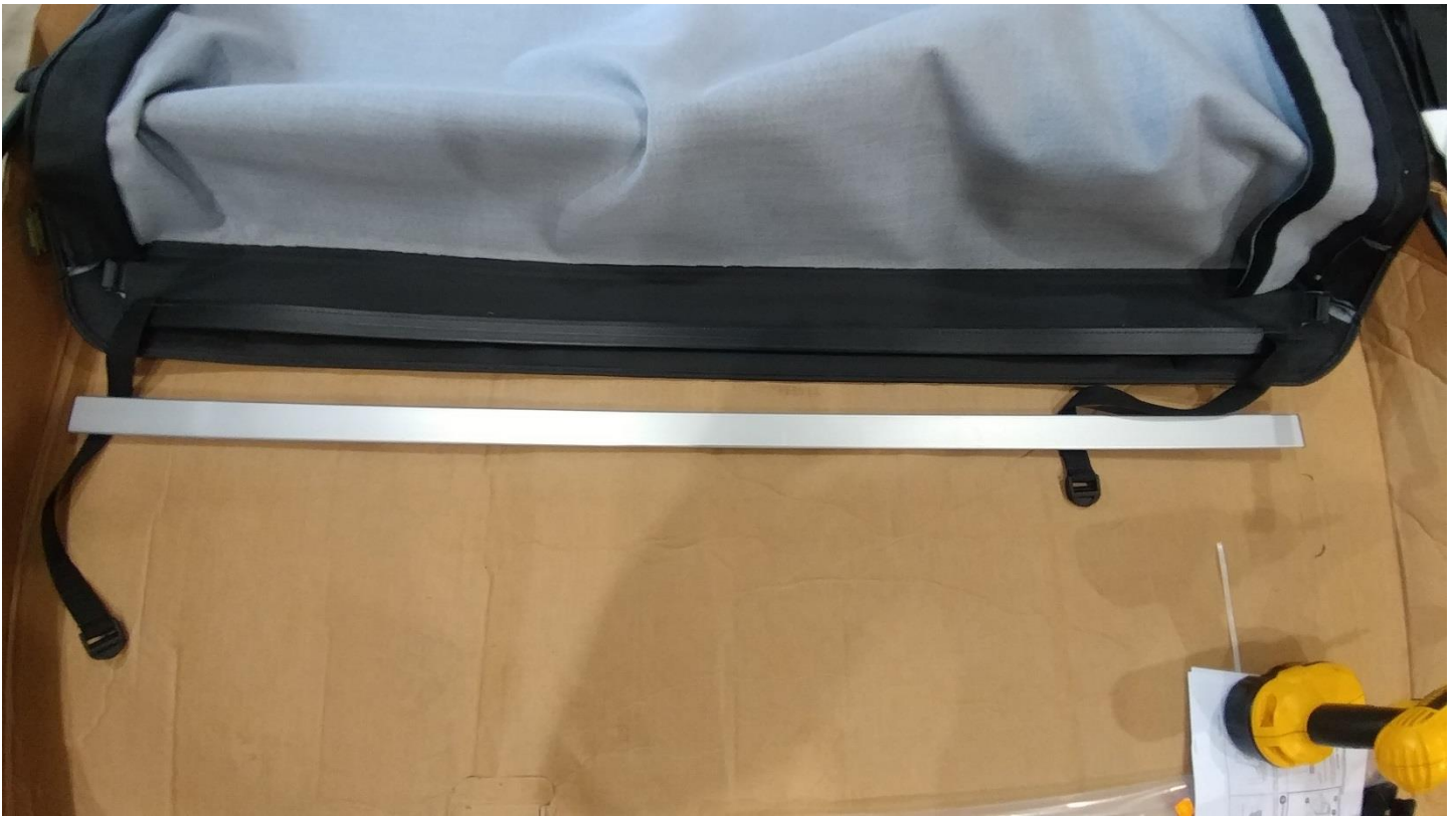
27. Insert the rear support bar into the pocket at the back of the cloth top
