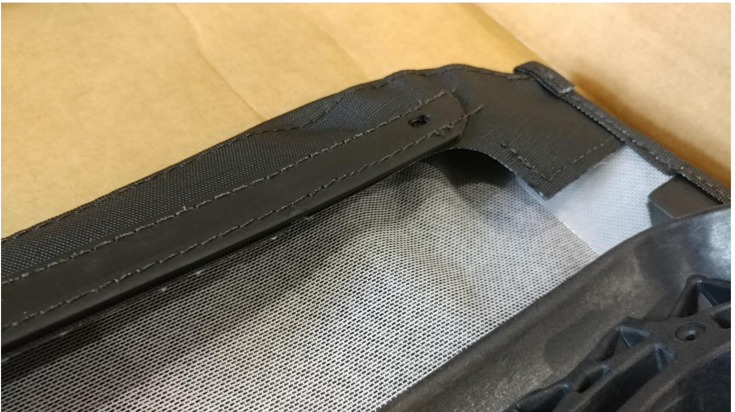
21. Starting with the center hole line it up with the pre-formed holes in the header
