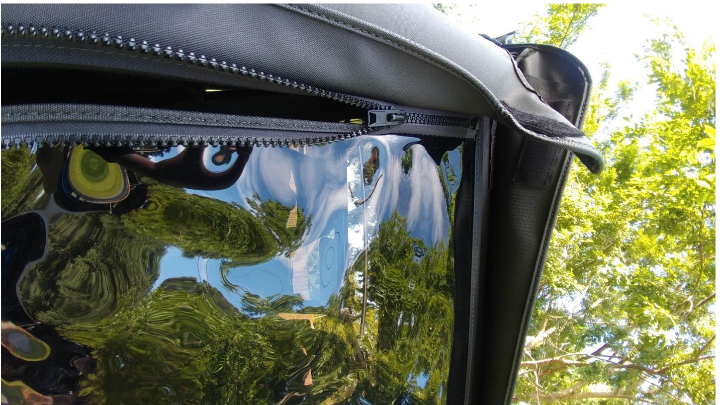
40. Insert the driver side window into the door surround
