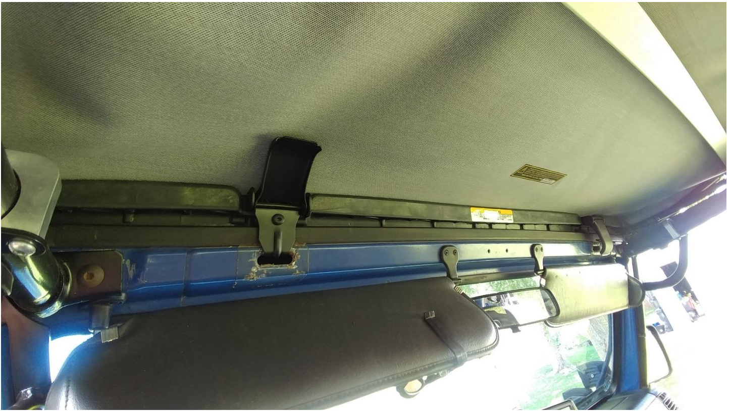
33. Secure the rear straps. Route the strap through the buckle as shown
