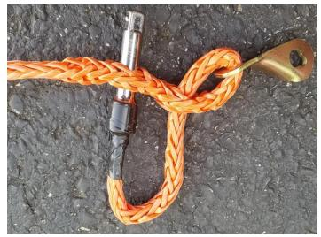
TIP: The tail can be secured by feeding it into itself.
