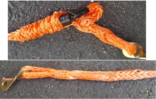
5. Slide the nylon sleeve back over the line to the metal connection link. **TIP:** A piece of nylon webbing can be used as a keeper to prevent the winch line from being pulled all the way out during use. This will allow the winch line to grab securely on the winch spool during use without risking breaking the winch from the spool.
