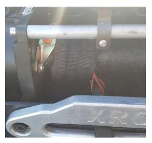
8. Winding the Winch line onto the spool should be done with tension on the line. This will prevent the Winch line from binding or pinching on itself during use. A secure point such as a tree or a pole can be used as an anchor point or a heavy object (such as another vehicle or lawn mower) can be used. Alternatively, the Winch can be wound by holding tension on the Winch line. This is not recommended since the line will be loose on the spool.
