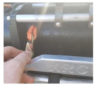
If using a keeper strap as noted above, loop the line around the spool 4 times but keep it loose. Then feed the keeper strap under the Winch line (between the line and the spool) and loop it over the end of the Winch line before securing the Winch line.
