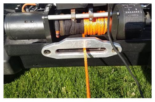
9. Install your choice of an end link system and secure the end of the Winch line to ensure it does not get hung up on anything.
