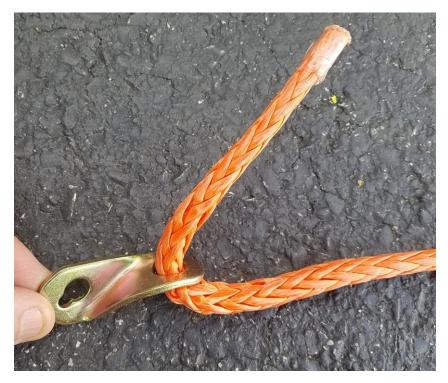
4. Pull enough line (approx. 1 ft) through the hole to work with. Feed the line back through itself to secure the line. When the line becomes tight, it will keep tension on itself. This is done bunching the line up to loosen the strands. **TIP**: A 3/8 socket extension can be used to help guide the rope through itself.
