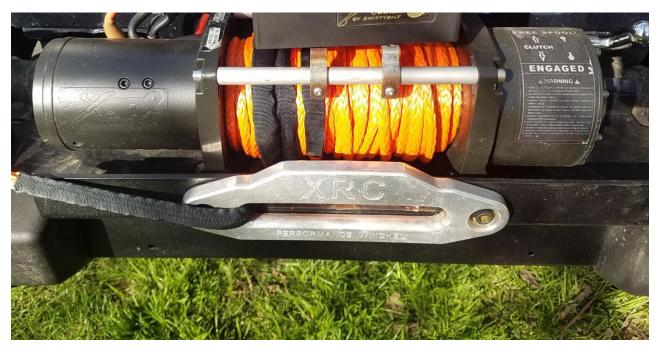
**NOTE:** Sun light will cause damage to the synthetic line over time. The line should be kept covered to prevent premature failure.
