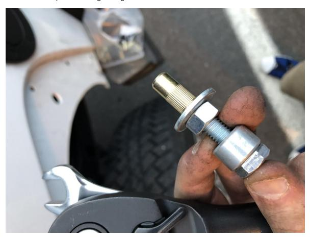
6. Inserted rivnuts should not be able to move and should look like the picture below when completed. (NOTE: one rivnut is different color as I cross-threaded the provided one and needed to replace it)
