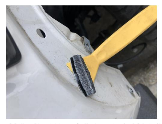
3. Apply provided rubber padding to inside upper edge of fenders, cut to length. Poke holes in rubber where mounting holes are to allow for easier bolt insertion.
