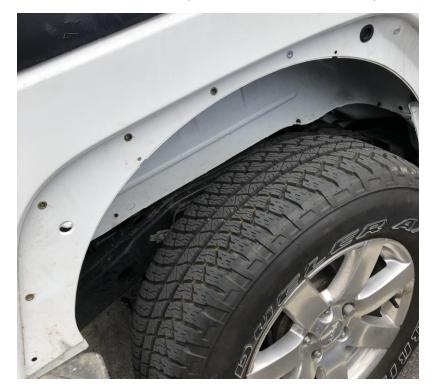
7. Align fender to mounting holes and use provided bolts and washers to mount. Loosely insert all bolts before tightening any. Locking washer should be located in between the head of the bolt and the regular washer. Tighten with 10mm socket.
