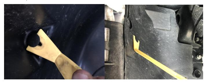
2. Lift up on fender and pull outwards with some force, fender clips should pop out of the frame, although some may break. Remove all fender clips still in the frame with the trim tool.
