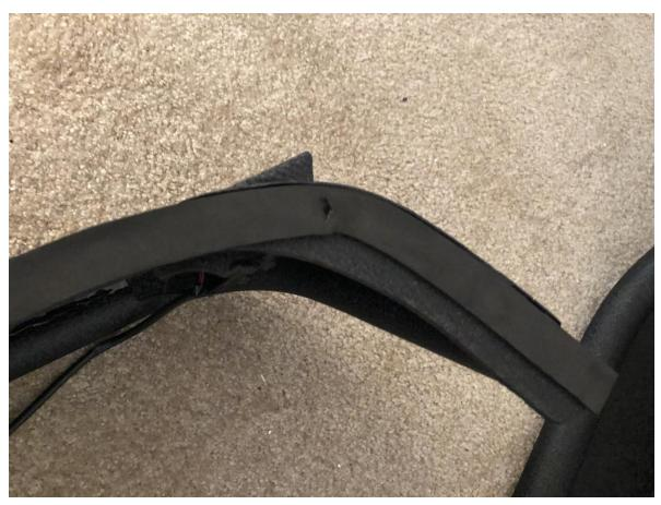
4. Use fender to verify which holes in frame will be mounted to by aligning mounting holes. All except the bottom on either side should be used. Mark these for easier identification.
