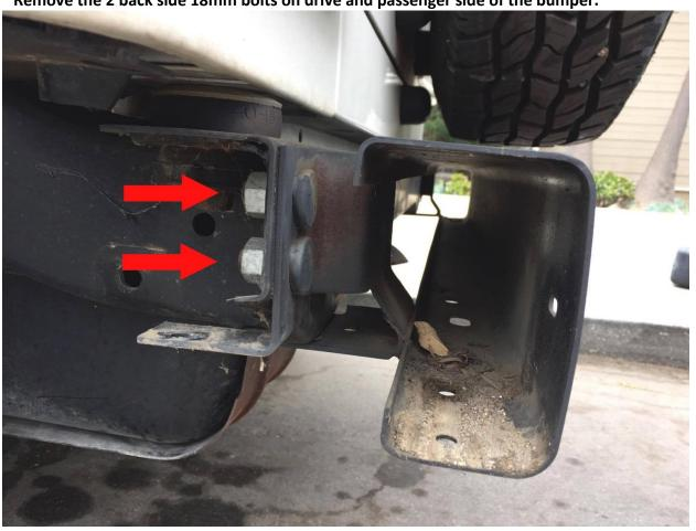
6. With the factory bumper removed, install the Barricade Trail Force HD Rear Bumper using the provided 6 - 18mm bolts. Use the original 6 holes for the factory bumper for the new Barricade Rear Bumper, 3 on each side.
