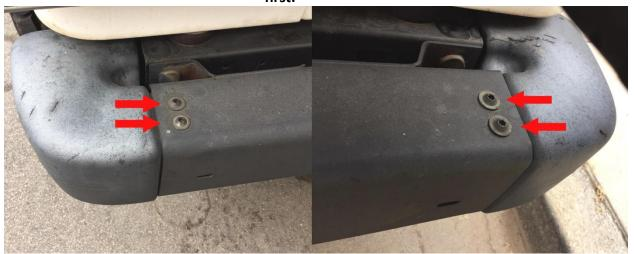
3. Remove the 3 bolts on each side of the bottom side of the bumper.
