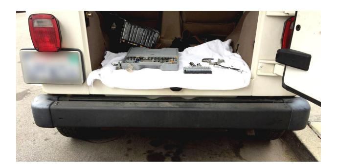
2. Remove rear bumper end caps using T30 Torx bit. There are 5 bolts on each side, 2 on the top side and 3 on the bottom side. Remove the 2 topside bolts on each side first.
