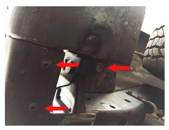
4. Remove 18mm bottom side bolt on the driver and passenger side of the bumper.
