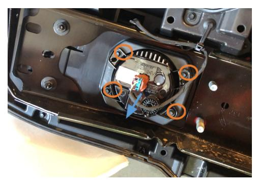
10. Mount fog lights to Trail Force bumper: use supplied machine screw and serrated face nuts to mount the fog lights to the trail force bumper. Notice the orientation of the fog light, the heatsink should be towards the top of the bumper
