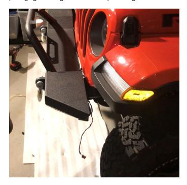
21. Plug wiring harness into both fog lights and vehicle harness.
