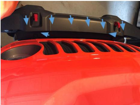
2. Remove lower splash guard: use a trim removal tool or a small screwdriver to remove pop-clips (blue) and then use a 8mm socket to remove the two screws securing the splash guard to the skid plate (orange).
