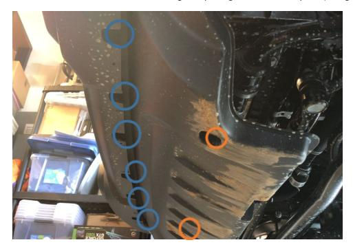
3. Remove side trim panels: use a trim removal tool or a small screwdriver to remove pop-clips
