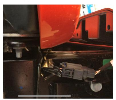
22. Zip tie slack to bumper support brackets, making sure not to stress connections.
