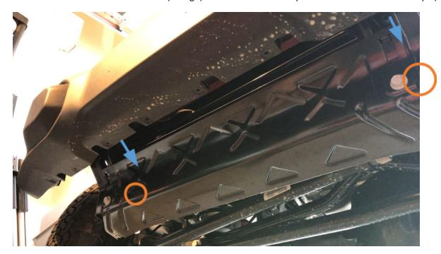
5. Unplug fog light harness: unplug the wiring harness from the vehicle by squeezing the clip (blue) then pulling it out (orange)
