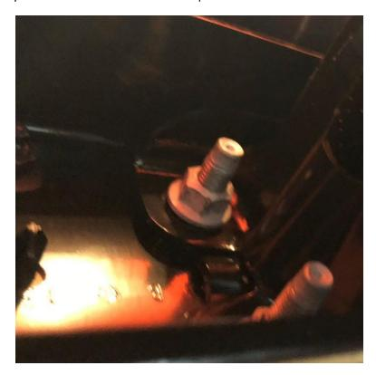
7. Loosen bumper support brackets (four): loosen the bumper support brackets nut but do not remove. Remove the brackets and put them to the side, keeping track of which bracket goes where.
