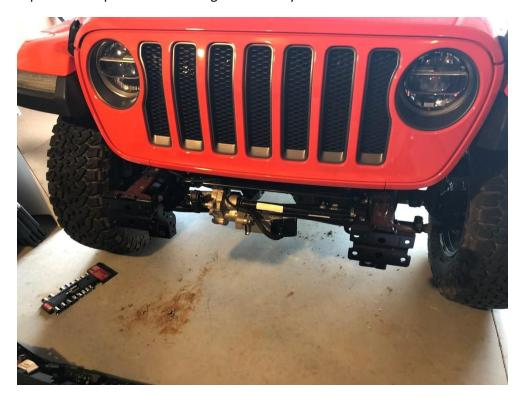
9. Remove fog lights: unplug fog lights from wiring harness and use 7mm socket to remove 4 screws from each fog light.
