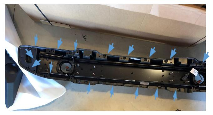
12. Remove wiring harness for fog lights: unplug fog lights from wiring harness, then use a trim removal tool or a small screwdriver to remove pop-clips
