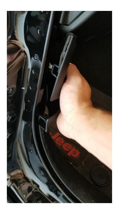
9. Secure mirror arm from Round Adventure Mirror package by placing the lock and nut on the threads of the arm after placing the arm through the top external door bracket. Securely tighten nuts with a 15 mm socket.
