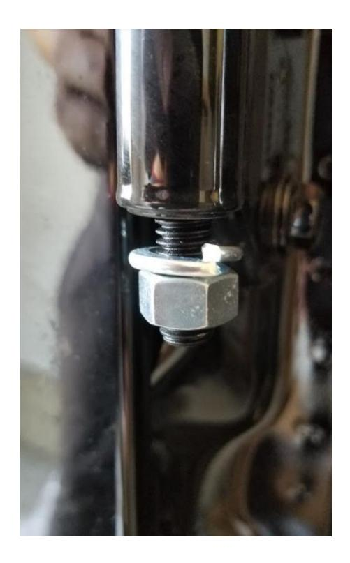
10. Secure the mirror by unscrewing the 13 mm bolt from the back of the mirror, and then placing the bolt through the eye of the extending arm in the previous step. Tighten securely. Ensure that the mirror does not fall off of the arm before the bolt is securely placed on the mirror.
