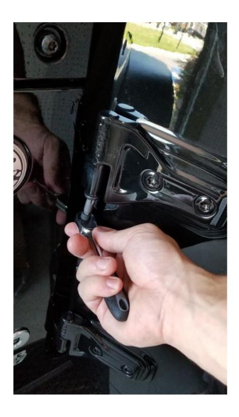
6. Securely store door jamb bolt and the two exterior bolts in the back of the vehicle under the cargo area.
