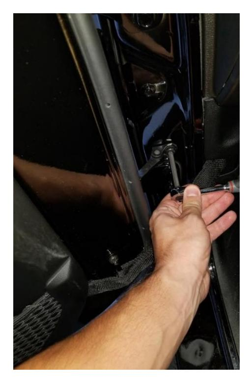
4. Disconnect wiring harness for the door by pushing down on the RED clip, then grasping the bottom black clip. This will allow you to push the white brace upwards. Continue pushing upwards until the wiring harness disconnects itself.
