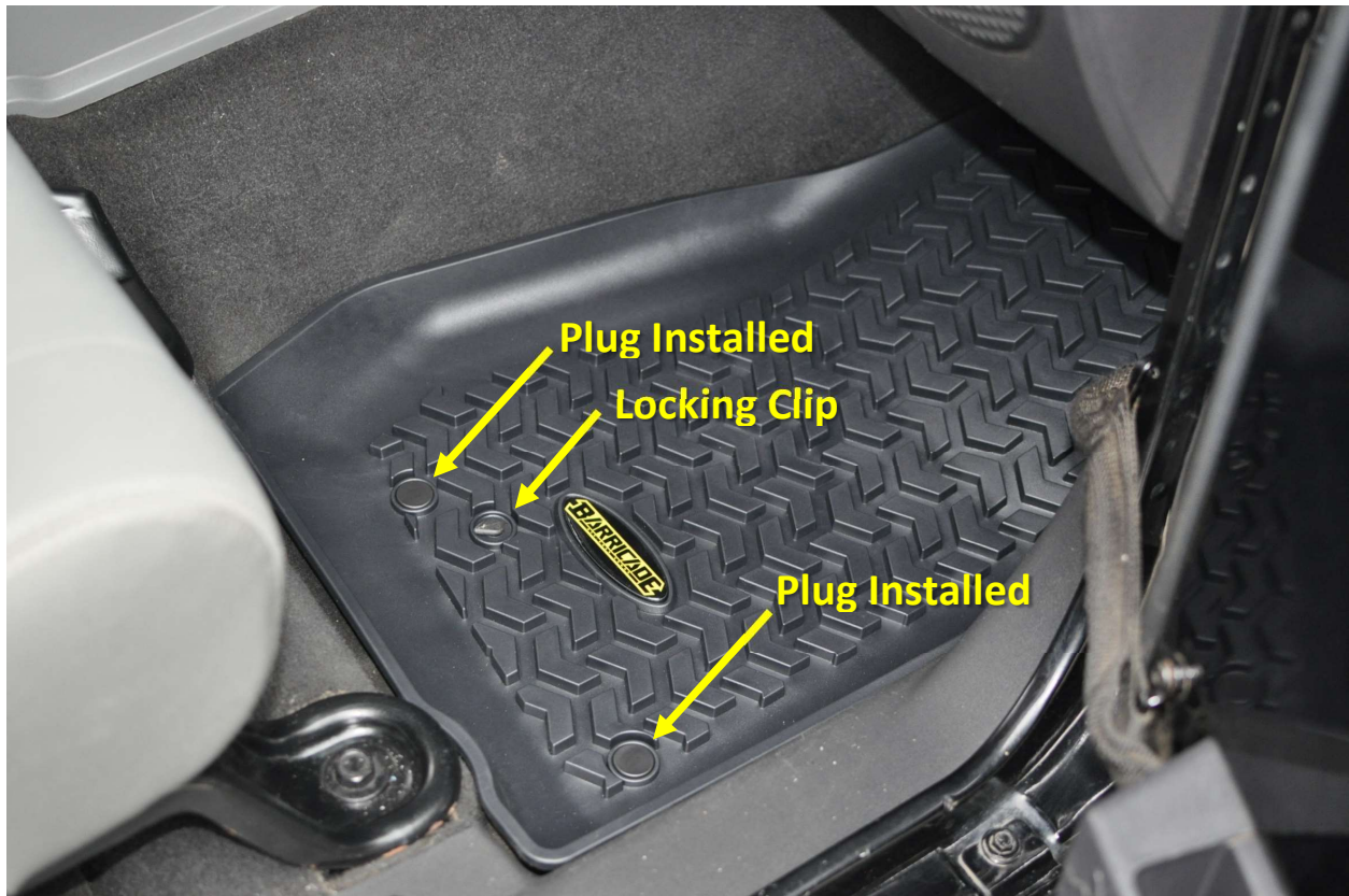
Passenger Side Installed:
