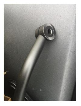
5. Place knurled link into bracket and tighten by hand securely. Adjust angle of bracket mirror as needed.
