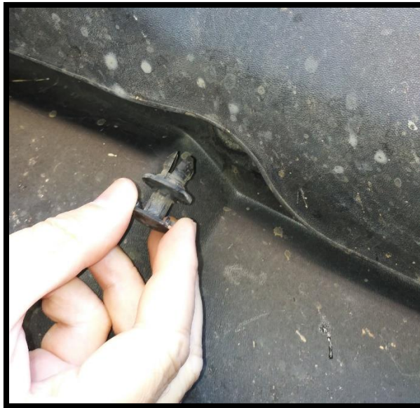
Plug removed from air dam
