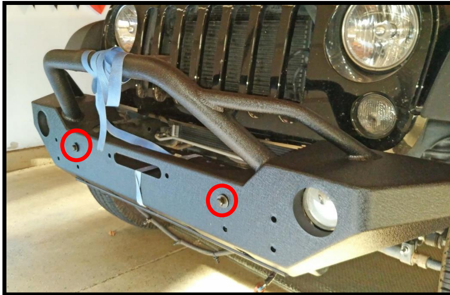
Bumper temporarily held in place with two bolts
