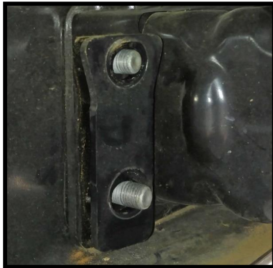
Bumper retaining plate after nut removal
