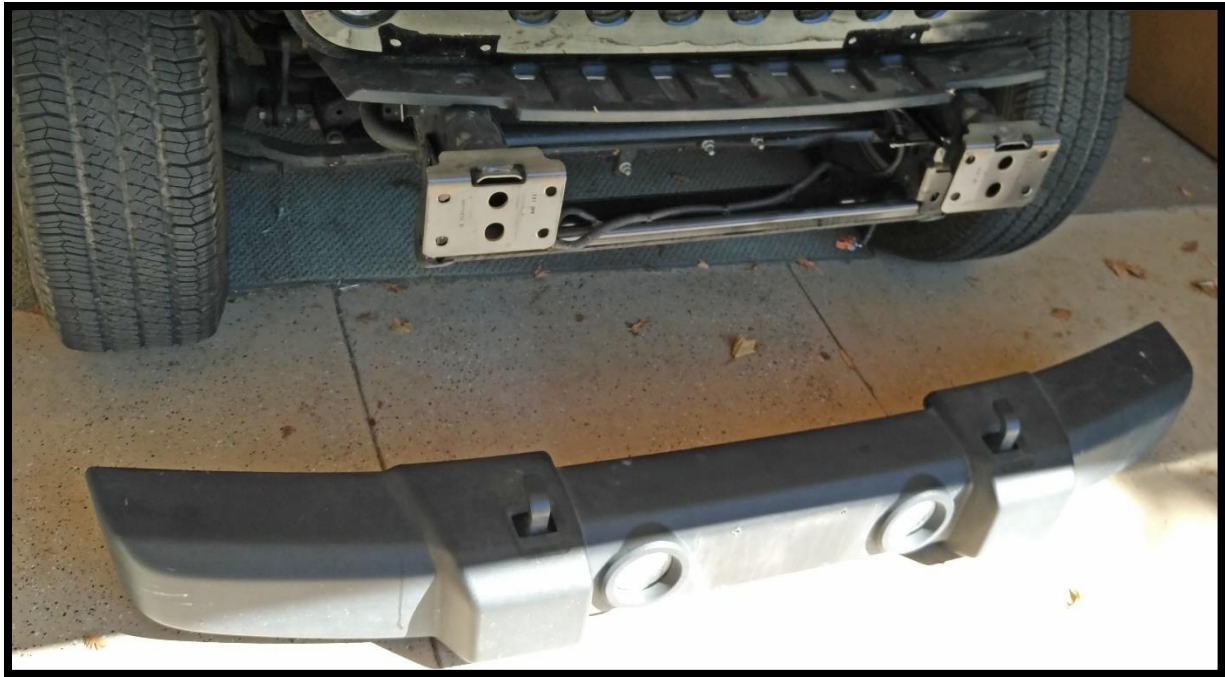
Bumper removed from frame. Notice the 8 holes which the bolts went through.
