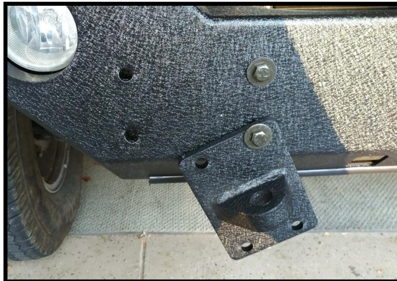
Shackle plate installation on passenger side
