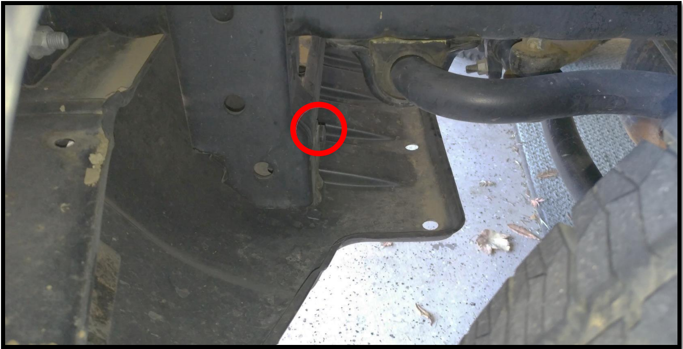
Rear Air Dam plug, driver side, there is also one on the passenger side.
