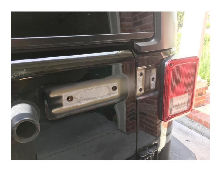
included kit bolts and 5mm allen wrench (Note: Do not fully tighten at this point to allow for adjustments; It is also recommended to use included anti-seize on these bolts when installing)
