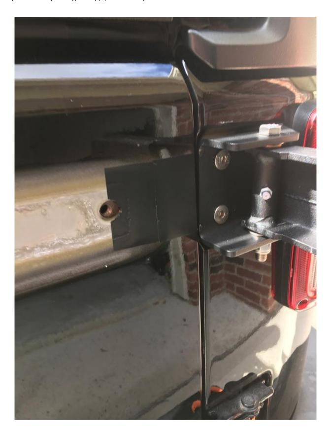
8. Attach heavy duty hinge to tailgate using bolts included in the kit and serrated lock washers with 13mm socket wrench and extension using anti-seize on bolts if desired (Note: Lock washers should be installed between bolt
