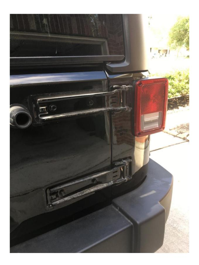
3. Remove two bolts connecting top factory hinge to tailgate using 13mm socket and wrench
