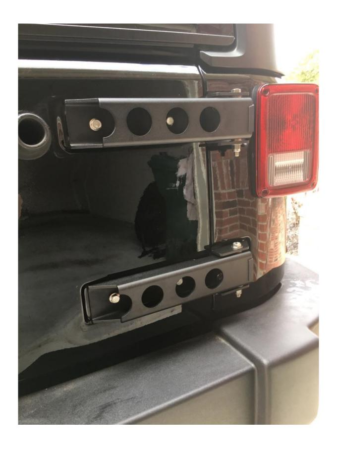
10. Adjust hinges so that the tailgate latches properly and the tailgate support mount below the latch lines up and helps to support the tailgate
