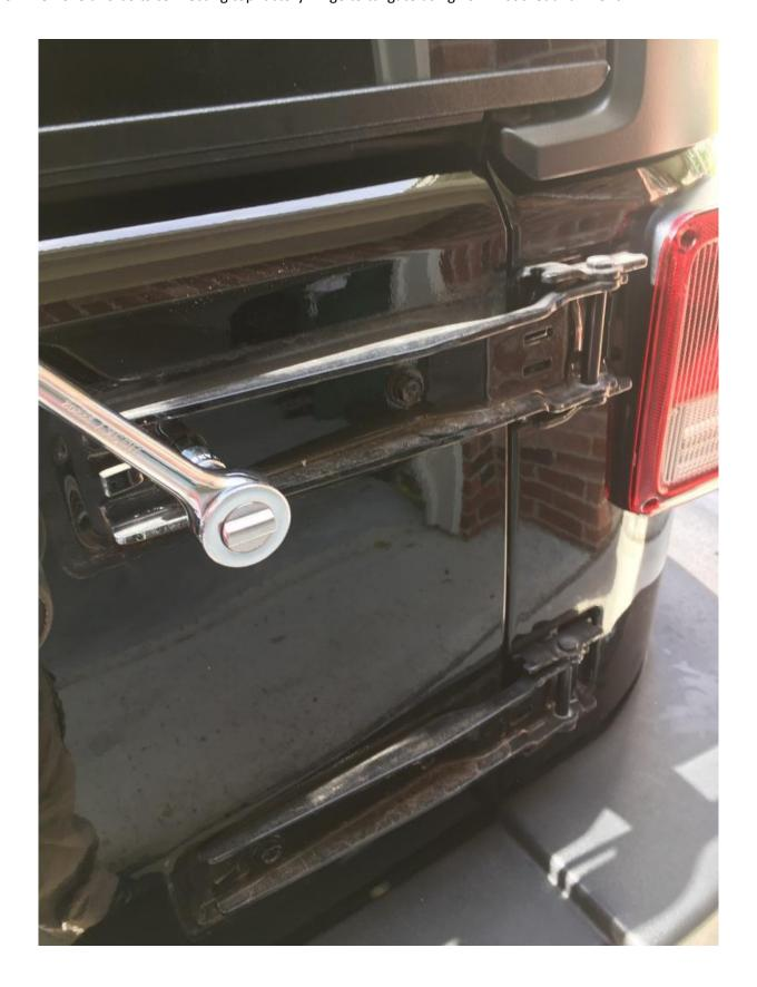
4. Remove three bolts connecting factory hinge to jeep quarter-panel using T-50 torx bit and wrench (Note: you
