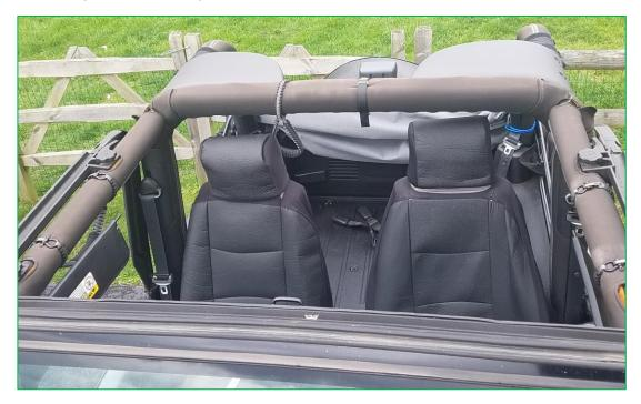
2. Attach center clasp to center latch over the windshield. Make sure the opening to the pockets are facing into the passenger compartment.
