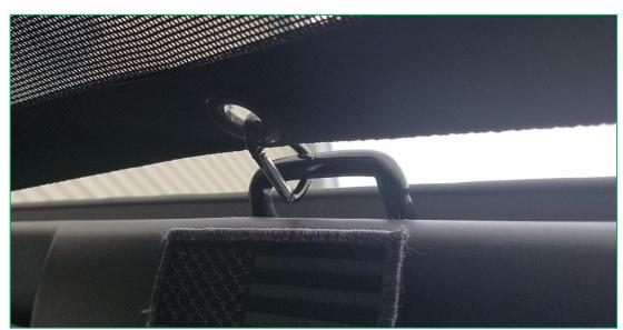
3. Starting on the driver side front, place the bungee cord through the eyelet with the ball facing the inside of the passenger compartment. Go over the roll bar (in front of the window surround Nut) and between the window surround and roll bar. Loop the bungee around the ball to secure the top.
