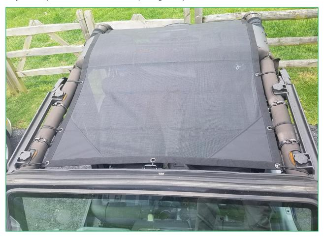
**Tip:** Use a zip tie to ensure the bungees remain secure around the ball. Do not over tighten the zip tie and trim the tail.
