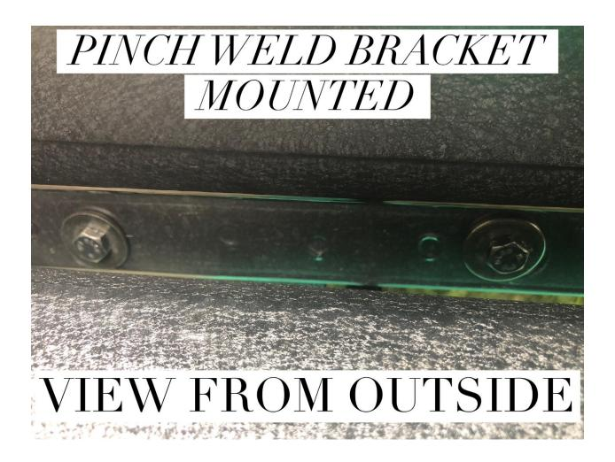
**Step 6:** After mounting all 3 pinch weld seam mounting brackets, the holes on the bracket and the holes on the steps should be aligned. Use the provided Hardware to attach the Pinch weld Mounting brackets to the brackets built into the steps. Make sure to use a washer on each side! Only hand tighten all nuts and bolts to allow for adjustment later
