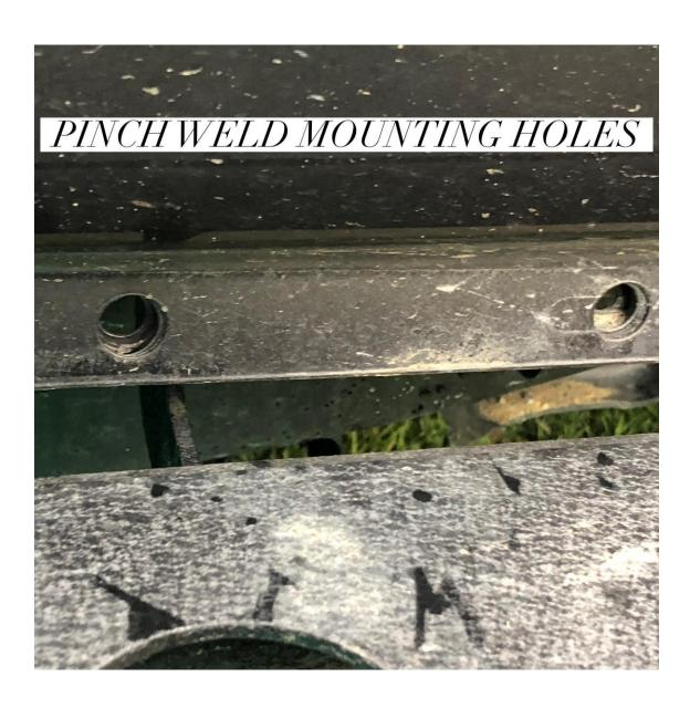
**Step 4:** locate the front bracket. The front bracket will have a small cutout to go around the "bulge" on the inside of the pinch weld seam. Hold up bracket under car and align pre drilled holes to holes on bracket. Bracket will be mounted on the inside edge of the pinch weld seam. Insert the 10mm bolt into holes from the outside so the threaded portion is under the jeep. Only hand tighten.
