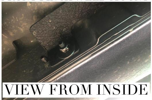
**Step 5:** After mounting the front bracket to the pinch weld, locate the other 2 brackets. You will have 2 identical brackets... one that will mount in the middle and one on the back of the steps. Follow mounting steps from **step 4** for both the middle and rear bracket.
