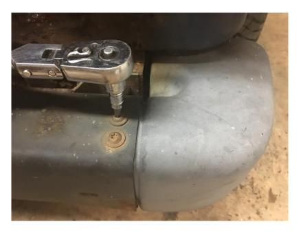
2. Remove the 18mm bolts that hold the bumper to the Jeep. There are 2 on each side.
