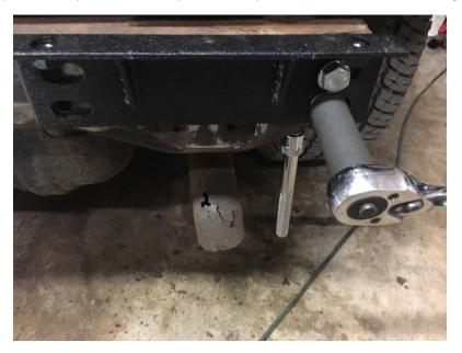
8. Once the mounting plates are installed, put the bumper on the mounting plates and attach the 4 supplied 18mm bolts. Then secure the bottom bumper tabs to the existing frame mounting holes with the bolts you removed when taking off the original bumper.
