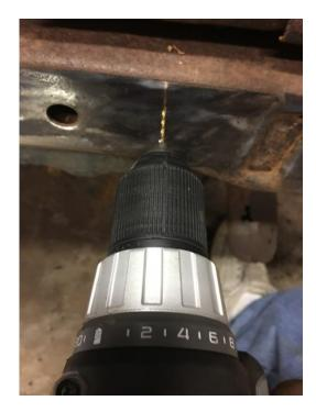
6. Once the pilot holes were drilled, I used a unibit to drill the holes to the correct size for the mounting bolts.
