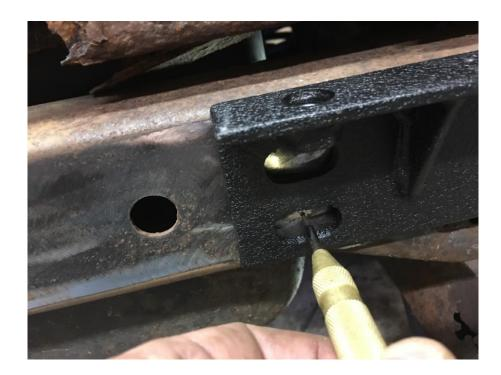
5. I then removed the mounting plates and drilled a pilot hole with a 1/8 drill bit. Be aware that the gas tank is right behind the holes you will drill so don't go too far once the bit gets all the way through. If you don't think you can stop before hitting the gas tank you can use drill bit collars.
