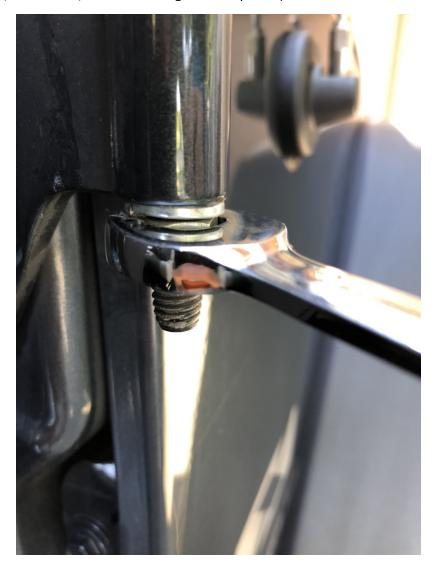
4. Adjust the mirrors so that you can clearly see out of them when sitting in the driver seat. (I Found it helpful to have someone adjust and tighten the mirrors into place while the driver of the vehicle sat in the driver's seat to make sure the mirrors where were they needed to be.
