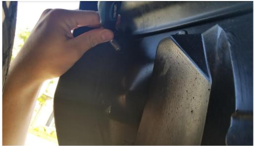
8. Disconnect the fog lights on both sides of the vehicle by grasping where the harness meets the fog light and pulling. There should be no tools required for this step.
