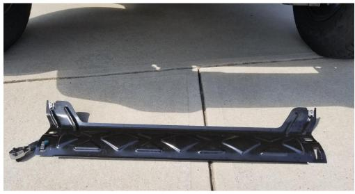
10. Remove the eight nuts (four on each side) on the studs holding the bumper on the vehicle. This should be performed on both sides of the Jeep using an 18 mm socket.
