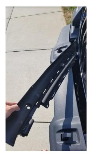
4. Remove lower splash guard. There are eight pop clips holding the splash guard into place. Using a flathead or your trim removal tool, remove the pop clips holding the splash guard.
