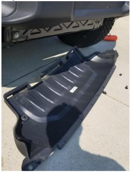
7. Remove the 7 mm screws holding on the caps to the bumper. There are 6 in total on each side. Repeat for the other endcap on the opposite side of the vehicle.
