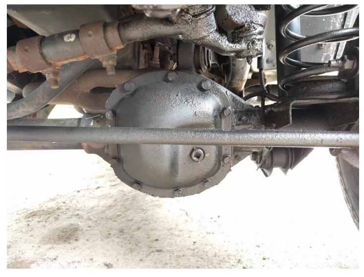
2. After placing drain pan under pumpkin, use ratchet or impact along with 1/2" socket and extension to remove all bolts except top one, then loosen top bolt. Firmly tap driver's side of existing diff cover with hammer/mallet to loosen or alternatively, insert screwdriver/putty knife to break seal and gently pry at bottom edge to loosen taking care not to damage inner surfaces. Allow gear oil to drain. Remove final bolt allowing cover to be removed.
