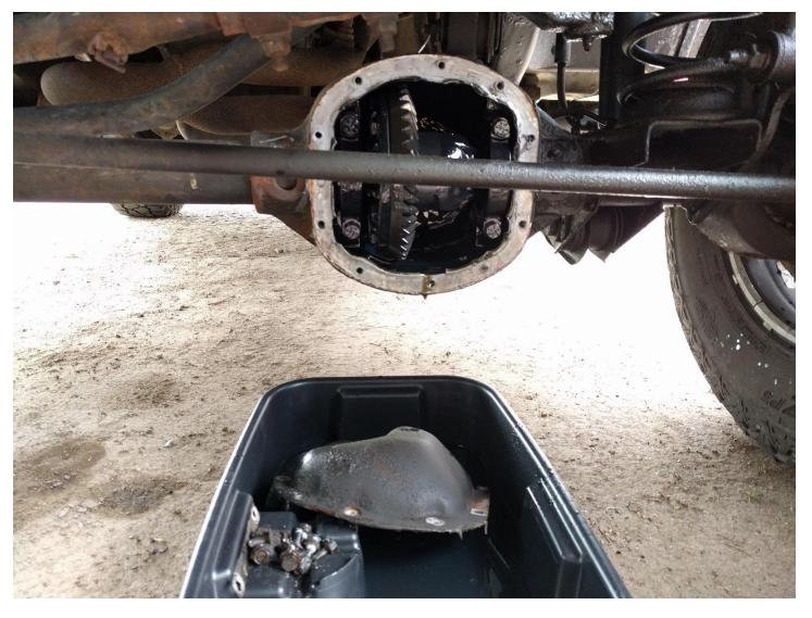
3. Carefully scrape any existing sealant to remove, again taking care to not damage mating surface. Cover gears with shop towel and spray housing liberally with brake cleaner. Recommended to polish mating surface with Scotch-brite pad or polishing wheel and additional brake cleaner as necessary.
