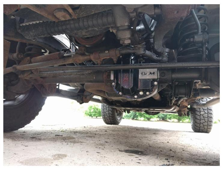
6. Fill differential with gear oil per vehicle spec. On Wrangler with minimal lift, top fill port on cover is easier to access by lowering Jeep off of jack/stands and using long funnel from inside engine compartment after temporarily moving coolant overflow tank out of the way. On lifted Jeeps/Other vehicles this may be easier to access under the vehicle at the fill port directly. Picture for reference in fill-port location.
