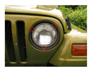
Step 2: Remove the 4 T15 Torx screws that hold the headlight bezel.
