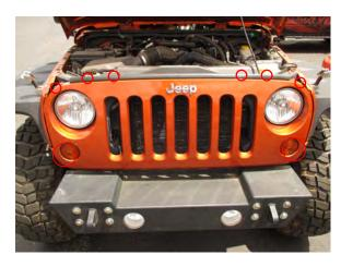
Step 2: Remove the 4 T15 Torx screws holding the headlight bezel.
