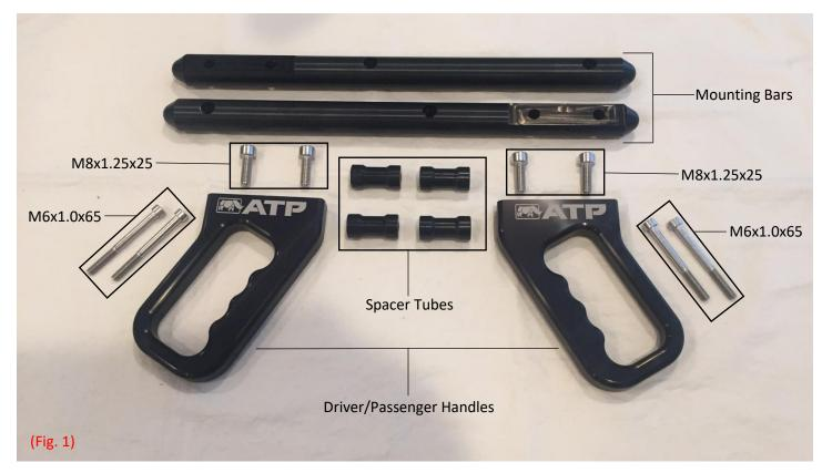
1. Preassemble both handles using the driver/passenger handles, mounting bars, and the M8x1.25x25 bolts with an H6 socket or 6mm hex key (Fig. 2).
