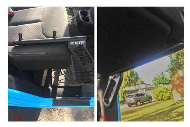
4. Tighten the M6x1.0x65 bolts by alternating from one to the other until both are tight and the handle is secure.
