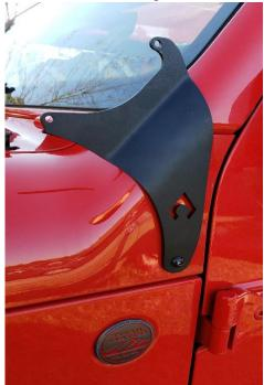
• Next you will install the top bracket using the 2 longer bolts and the 4mm Allen key. Make sure everything lines up before completely tightening the bolts.
