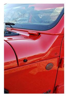
• Start by removing the 3 factory bolts from your cowl with the T-40 torx bit. There are 4 bolts total on the cowl, but only remove the top 2 and the 1 on the side that is located closer to the door. These are you mounting points for the new hardware.
