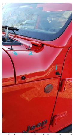
• Now simply drop the spacers in the appropriate holes and attach the side piece to the apillar with the included bolt (shorter bolt) and tighten with the 5mm Allen key.
