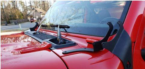
• Note that you do not need to fully tighten all of the bolts until you have added your lights in so that you have a little wiggle room to get them where they need to be. The mounting width for lights to work with this bracket is between 1.93-2.17" apart. That is around a 3-inch light, so make sure you get the correct size light to go with this.
