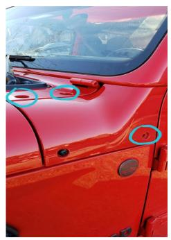
• The included bolts are all the same length, but there are 3 different size spacers that will be used. They are identified by have 1 groove, 2 grooves, and 3 grooves in the sides. The single groove is used on the lower bolt, the double on the top located closer to the windshield, and the triple is used on the top further out. I have them labeled bellow with which spacer they correspond to.
