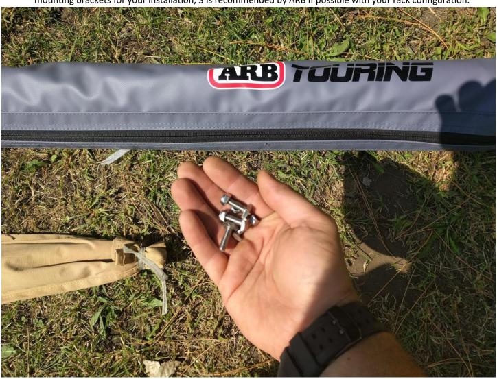
2. Prestage Bolts at the approximate mounting points/spacing in the aluminum track on the backside of the awning. This makes it FAR easier to install this without a second set of hands. OPTIONAL: Recruit a helper for the next step.
