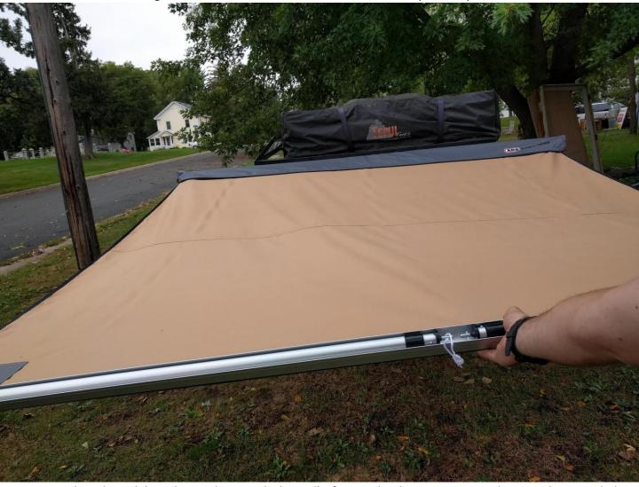
5. Now drop the stabilizing legs and twist to lock. Finally, from under the awning, secure horizontal arms with the attached velcro straps along sides.
