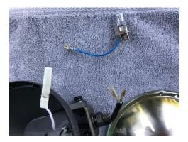
d. Replace the 55W bulb with the 100W bulb, reinstall the retaining wire, making sure the wire is in the grooves and plug in the 100W bulb.
