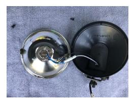
c. Lift the retaining wire up and out of the way and while holding the base, remove and unplug the 55W bulbs at the quick disconnect.
