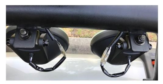
6. Ground the short black wire from the lights to a suitable body ground.
