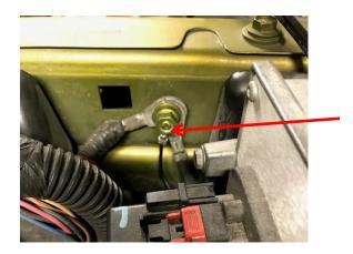
10. Route the yellow fused wire to the battery and install the wire connector to the (+) accessory post and tighten to 62 in-lbs with a 10 mm wrench.
