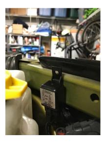
8. Ground the relay to a body ground post.
