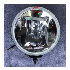
b. Removed the (2) screws holding the reflector/lens into the light body.
