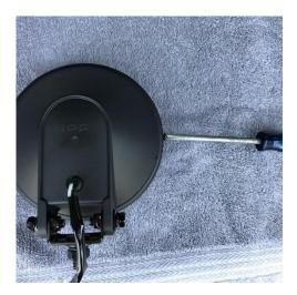
b. Remove the reflector/lens assembly from the body.
