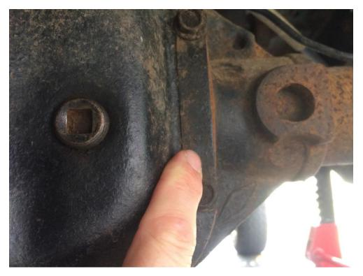
6. Apply gasket maker or gasket according to manufacturer directions to new cover and install using supplied bolts and washers. Thread all bolts in loosely by hand before tightening. Do not over tighten. The factory recommended torque values might be too high for this hardware.
