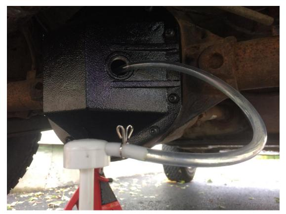
8. Replace fill plug. Tighten with supplied 12mm hex wrench.
