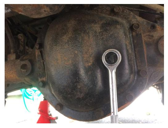
2. Loosen and remove differential cover bolts using ½ inch socket. You may find it helpful to leave a top bolt in place to avoid dropping the cover as you remove it. The old cover may be stuck in place. If so hit it with a large hammer to break it free.
