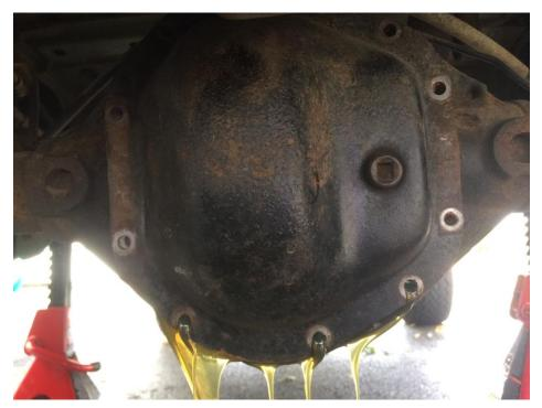
4. Clean and dry mating surface of differential and differential cover well. Remove old sealant or gasket as needed. Inspect gears.
