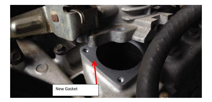
3. Next place the new throttle body spacer on top of new gasket, making sure its facing the right direction. It should say "top 4.0."
