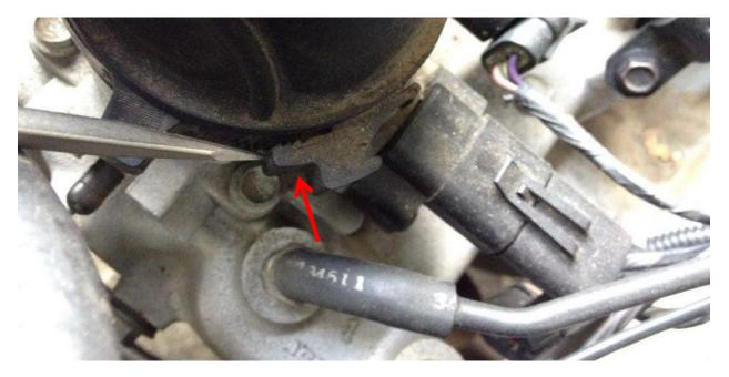
2. Next remove the four 10mm bolts from the throttle body. Lift up on the throttle body and place the new (gasket) underneath. The new throttle body kit should come with two new gaskets.
