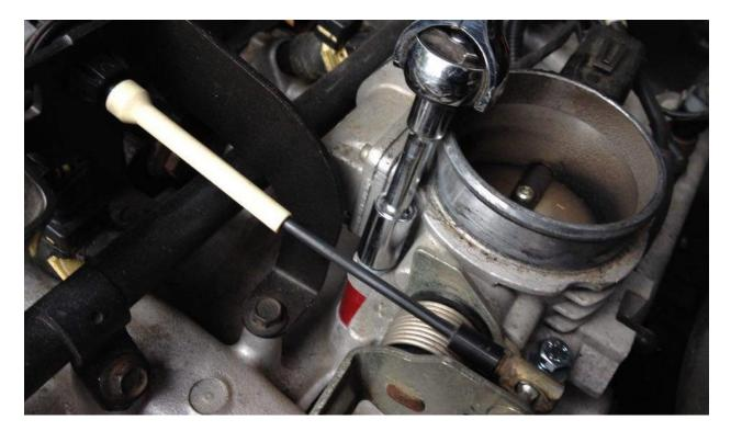
5. Make sure you operate the throttle cable, to ensure that the throttle plate isn't binding and there are no pieces of the gasket sticking out, restricting airflow.
