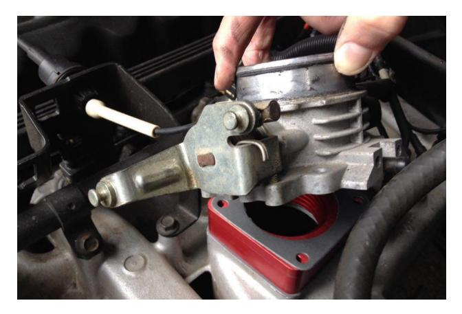
4. Install four new bolts with a ¼" ratchet and a 10mm ¼" socket. Tighten until snug, then ¼ turn.
