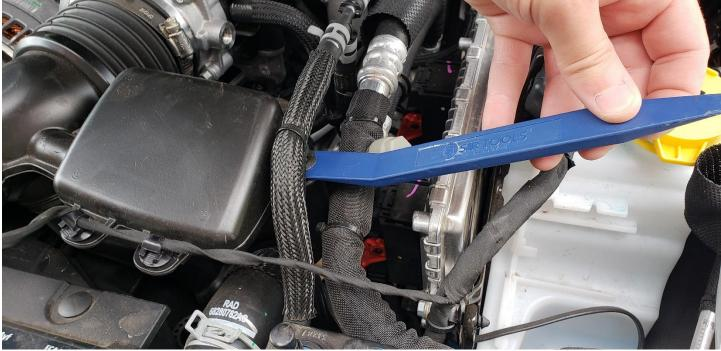
5. Disconnect the Crank Case Vent (CCV) connector from the top of the intake tube by holding down the large release tab and gently pulling back on the CCV line.
