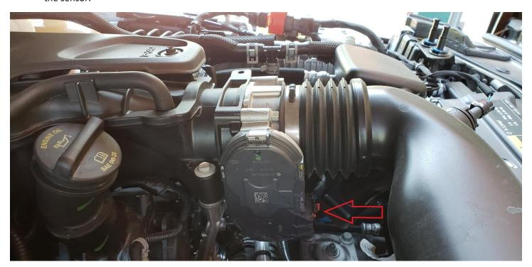
4. Using a panel popper tool, remove the two temp sensor harness clips and the one coolant line clip that are attached to the side of the intake tube.
