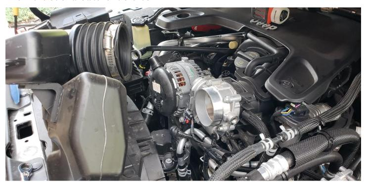
7. Remove the four bolts from the front of the throttle body using an 8mm socket and driver. Make sure not to let the throttle body hang by the wire harness after the screws are removed. NOTE: Do not discard factory hardware in the event vehicle must be returned to stock.
