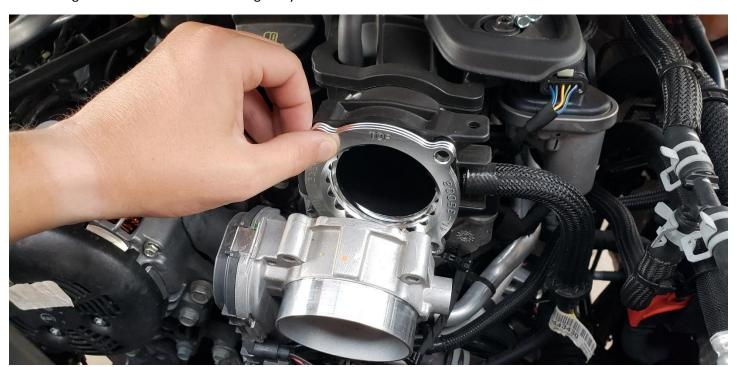
9. Place the gasket on the engraved side of the spacer and position the throttle body over the top of the gasket/spacer in the same orientation as it was originally. Using the new hardware and an 8mm socket and driver, put provided screws and washers into each of the four holes and tighten them by hand. CAUTION: INTAKE MANIFOLD IS PLASTIC! DO NOT OVERTIGHTEN SCREWS!
