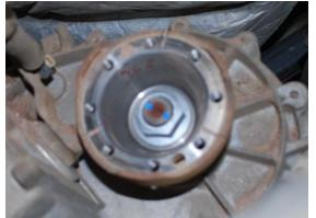
8. Using a puller, remove yoke. If you do not have a puller, you may be able to tap the yoke off with a small hammer, but be careful. Gently remove O-ring from old yoke and install in new yoke.
