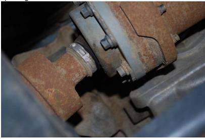
5. Using a 15 mm socket, unbolt the front of the driveshaft at the front differential. Retain these bolts as they will be reused with the new driveshaft. With the help of a friend, support the driveshaft on both ends, and fully unbolt the rest of the bolts from the front and rear of the driveshaft.
