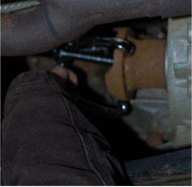
9. Gently place new yoke in place where old one was, making sure the splines line up easily. Put RTV on the yoke nut and reinstall. Tighten to 160 ft-lbs.
