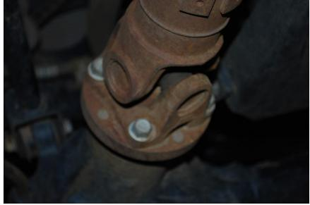
6. The rear end of the driveshaft may not separate easily, so you may need to gently pry it apart from the yoke using a large flathead screwdriver and hammer or awl. Carefully remove the driveshaft and set aside. You will find small indentations for an awl at the end of the yoke (see pictures).
