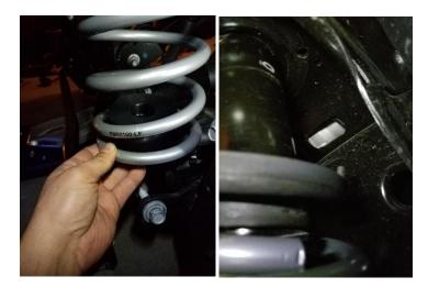
21. Rotate the coil springs so the end of the coil sits properly in the factory isolators and use a 14mm socket and wrench, secure the lower bump stop using the hardware supplied in the kit (HWC15057). Perform this step in the driver (shown) and passenger sides.
