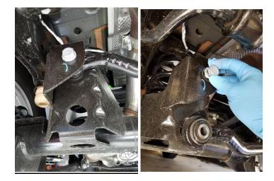
2. Using an 18mm wrench and socket, remove the screws securing the lower end of the links to the axle. Keep the factory hardware in the axle as these will be reused when installing the longer links. Perform this step in the driver (shown) and passenger sides.
