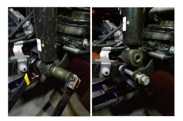
7. If you will install new shocks along with the lift, proceed to remove the bolt on the upper mount of the shock, and discard the stock shock responsibly. If you will keep the existing shocks and use a shock extension instead, you can keep the upper bolt and shock installed.
