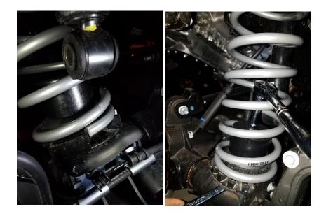
15. Using a 10mm socket, re-install the break and ABS lines bracket from the base of the coil spring previously removed from the passenger's side.
