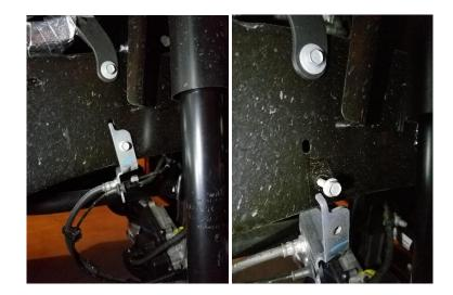
10. Using a 10mm socket, remove the break and ABS lines bracket from the base of the coil spring (only the passenger's side needs to be removed). This will allow to install the bump stop at a later step.
