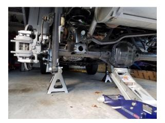
5. Using an 18mm socket, remove the nut securing the upper end of the links to the sway bar. Keep the factory hardware in the sway bar as these will be reused when installing the longer links. Perform this step in the driver (shown) and passenger sides.
