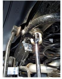
6. Using an 18mm wrench and socket, remove the screws securing the lower end of the shocks to the axle. Keep the factory hardware in the axle. Perform this step in the driver (shown) and passenger sides. If new shocks will be installed with this kit, remove the upper screw and remove the shock. Otherwise, the shock can remain attached to the frame as shown below.
