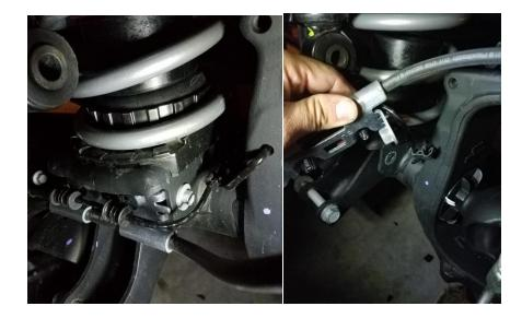
11. On Rubicon models only, remove the electric locker plug located in the front axle differential. There are two brackets attaching the wiring harness to the upper control arm and the frame (driver's side). Remove these with the pry tool.
