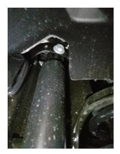
8. Using a 15mm socket remove the nut securing bracket holding the break and ABS lines attached to the lower control arm. Keep the hardware in the control arm. Perform this step in the passenger (shown) and the driver sides.
