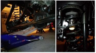
14. Once the axle is lowered and the springs have enough clearance, you can lift the spring towards the upper spring bucket and pull it out from the bottom. The rubber isolator from factory will be reused when installing the new coil spring. Perform this step in the driver (shown) and the passenger sides.
