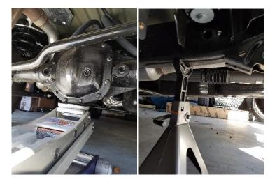
4. Remove the rear wheels and keep the jack in place supporting the axle.
