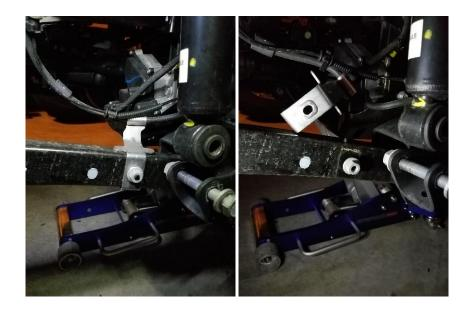
9. Using a 10mm socket remove the nut securing bracket securing the break and ABS lines to the frame. Once again, keep the hardware in the frame.
