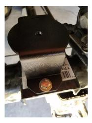
11. Now the new springs can be installed. Position the spring with the small diameter end facing up. Place the factory isolator sitting properly in the higher end of the coil spring. Ensure the index in the factory rubber is properly inserted into the hole on the upper spring bucket. Perform this step in the driver (shown) and passenger sides.
