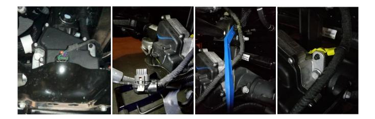
13. Using the floor jack, carefully lower the front axle. As the axle comes down, pay attention not to over-extend the break lines and the axle vent. Also make sure that the axle is not pulling on any lose parts (e.g. the disconnected wiring harnesses). Go as low as you can without over extending the break lines and vent. In this step the rear coils will separate from the upper spring bucket. Remove the factory coil springs from both the driver and passenger's side.
