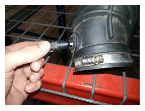
**6.** Install the IAT sensor into the new intake tube assembly.
