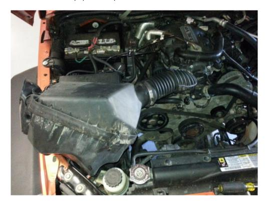
**5.** Remove your factory IAT sensor from the factory intake tube.
