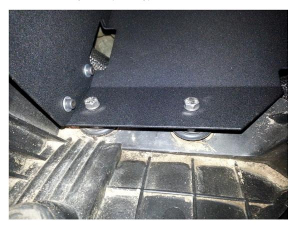
**10.** Add the supplied rubber gaskets to the top of the heat shield and in hole for the intake.
