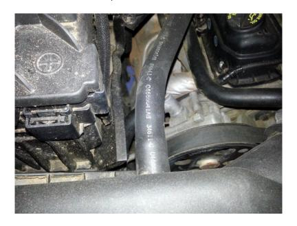
**3.** Using a flathead screwdriver, remove the hose clamp holding the intake tube to the throttle body.
