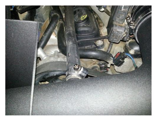
**14.** Plug in the IAT sensor that you previously installed into the intake tube.
