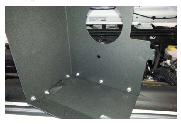
**8.** Remove the 8mm screw holding the fan shroud to the radiator.
