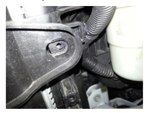
**9.** Install the heat shield using the factory mounting positions and secure with bolts.
