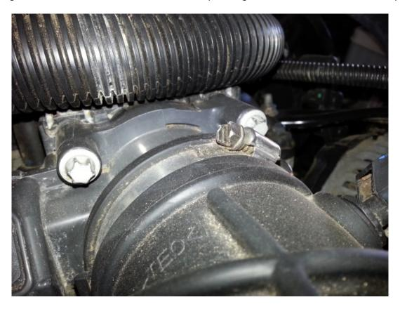
**4.** Pull the entire intake assembly up and away from the vehicle.
