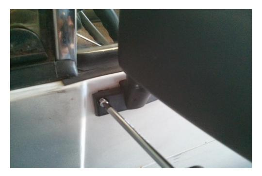
4. Install the cover plate. Note: attach the bottom of the cover plate first then lock the top plastic tabs into place.
