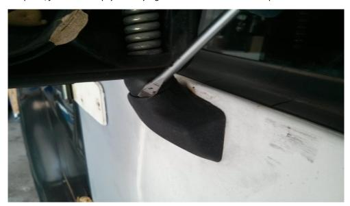
2. Using a Philips Head screwdriver remove the two sheet metal screws that secure the mirror to the door. (If screws appear rusted or damaged apply a good penetrating oil to the screw heads before attempting to remove the
