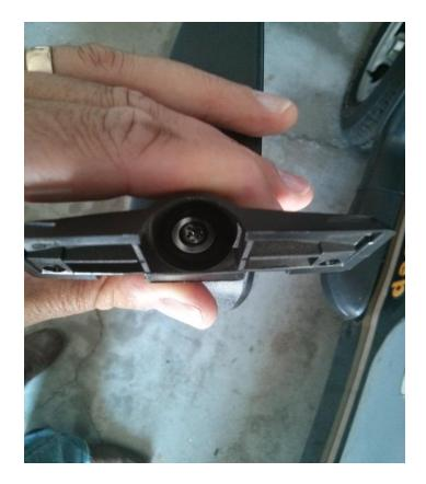
3. Using the supplied mounting hardware/screws attach the new mirror to the door.
