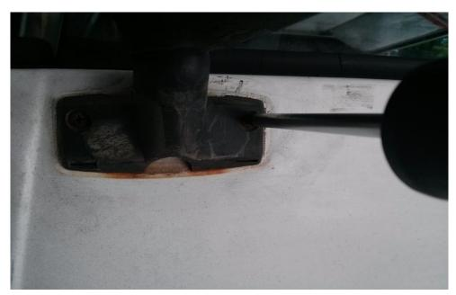
3. Clean the surface and remove any loose rust and dirt before installing the new mirror.
