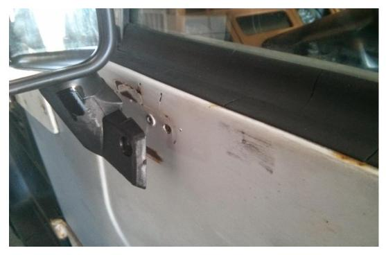
2. **IMPORTANT!** Before mounting the new mirror; adjust the tension screw located on the base of the mirror to ensure adequate tension to prevent the mirror from coming out of adjustment while driving on rough roads or rugged terrain.
